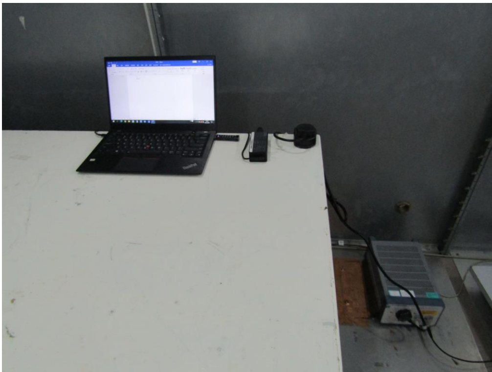
Measurement of Conducted Emission Test Set Up
