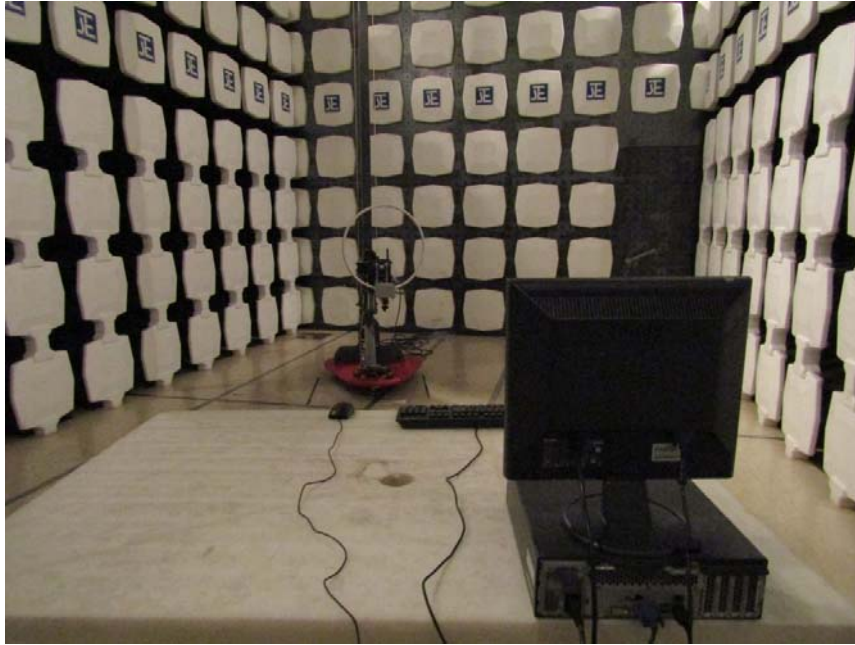
Measurement of Radiated Emission Test Set Up
