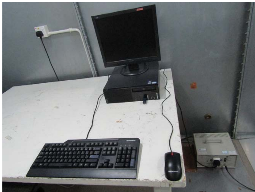
Measurement of Conducted Emission Test Set Up
