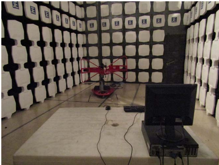
Measurement of Radiated Emission Test Set Up
