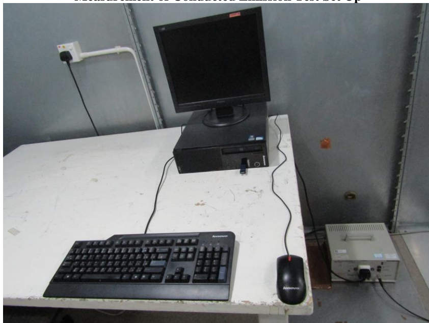
Measurement of Conducted Emission Test Set Up
