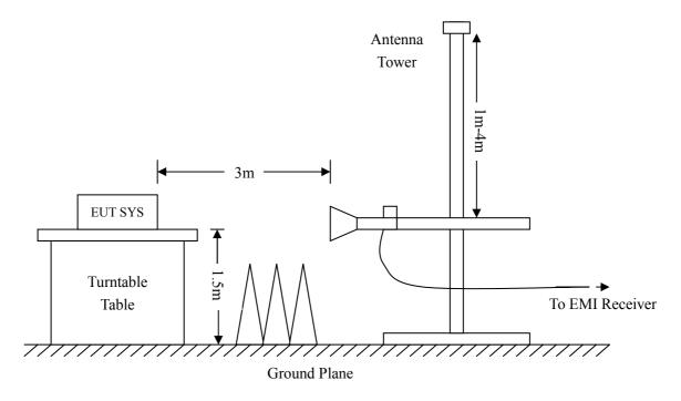
Frequency:9kHz-30MHz Frequency: Above 1GHz Frequency:30MHz-1GHz RBW=10KHz, RBW=120KHz, RBW=1MHz, VBW = 30KHzVBW=300KHz VBW=3MHz(Peak), 10Hz(AV) Sweep time= Auto Sweep time= Auto Sweep time= Auto Trace = max hold Trace = max hold Trace = max holdDetector function = peak Detector function = peak, QP Detector function = peak, AV
