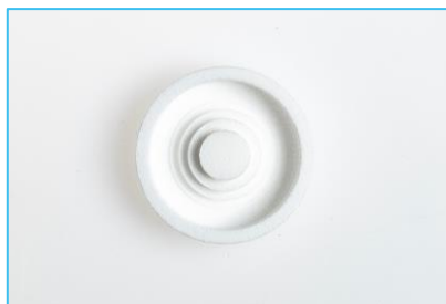
Figure 2.5. FZP lens diameter 36.3 mm and height 7.8 mm
