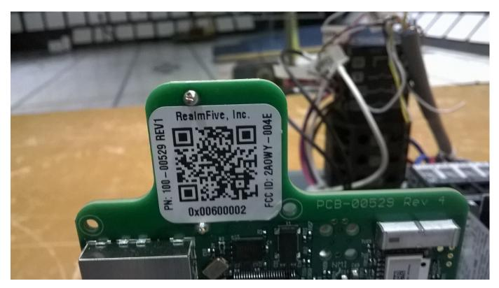
Label is thermal printed indelibly on vinyl material that is intended to last the lifetime of the device.
