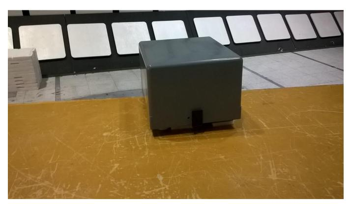
The device is typically installed within another sensor, but is itself a stand-alone transmitter that is capable or operating by itself with no sensor. The EUT was tested inside a representative enclosure, but the enclosure was all plastic and had negligible effect on test results.
