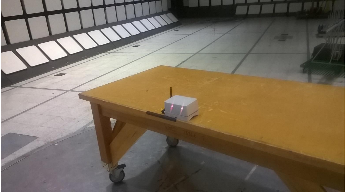
Figure 4 - Test setup for 30MHz - 1GHz
