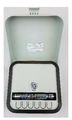
Open device lid to expose the unique device QR code.
