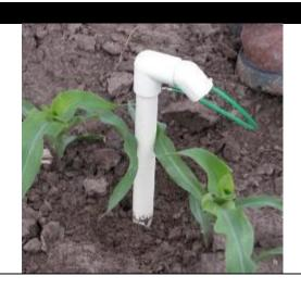
2.2 Install Sensor Integration Device on a 5' length of the same 3/4" CPVC post as the probes by pushing and twisting.
