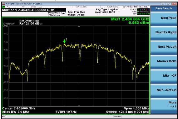
**Power Spectral Density Test Plot (CH-Mid)**
