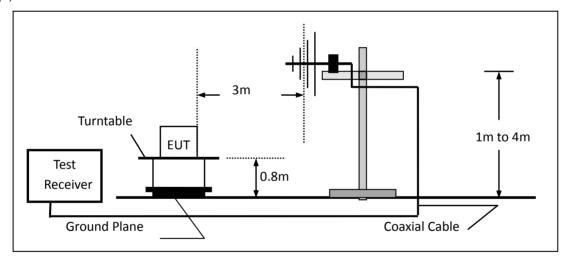
(c) For radiated emissions above 1000MHz
