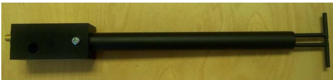
Figure 1 – MVG COMOSAR Validation Dipole
