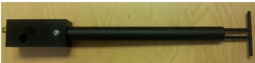
Figure 1 – MVG COMOSAR Validation Dipole
