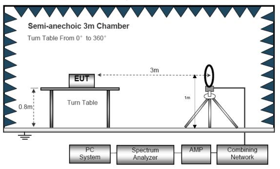
(B) Radiated Emission Test-Up Frequency 30MHz~1GHz
