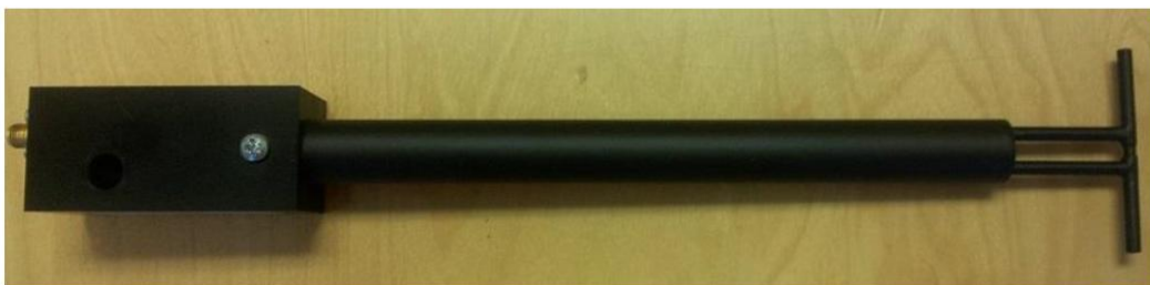
Figure 1 – MVG COMOSAR Validation Dipole
