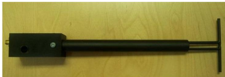
Figure 1 – MVG COMOSAR Validation Dipole
