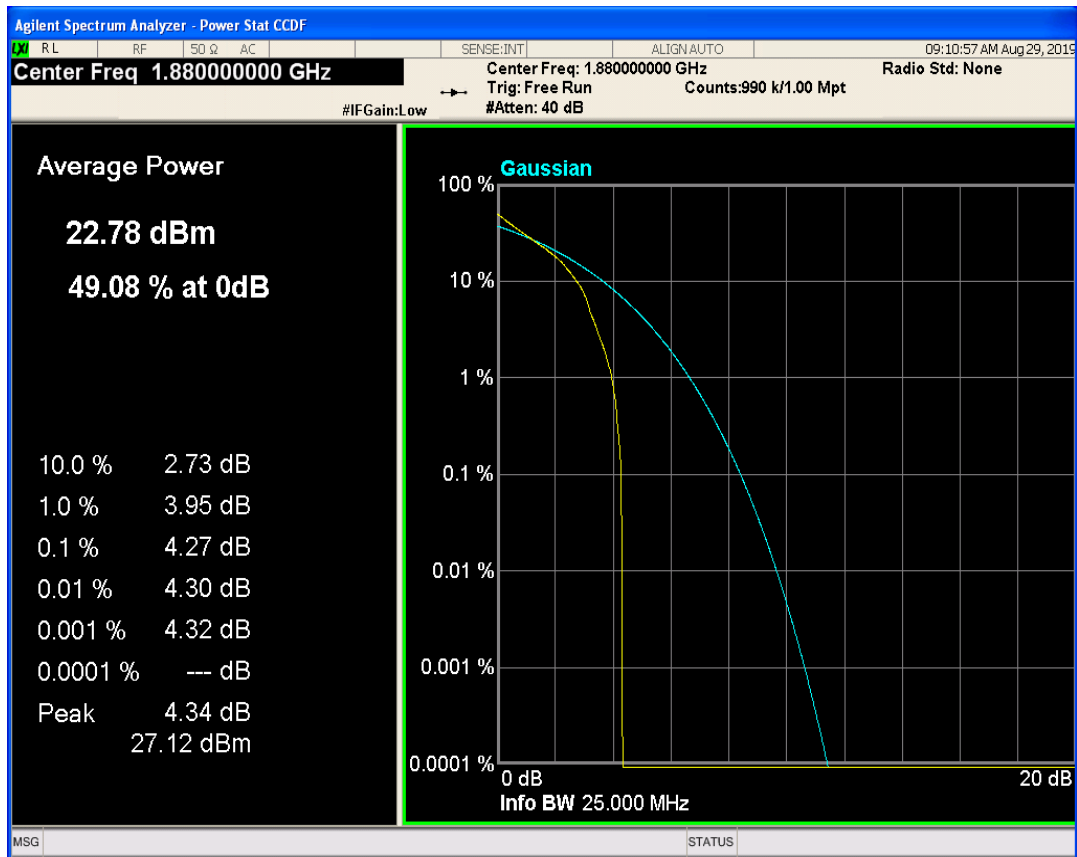
LTE Band2 QPSK BW=1.4MHz Channel=18900 RB Size=1 Position=#0
