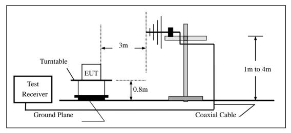
(c) For radiated emissions above 1000MHz
