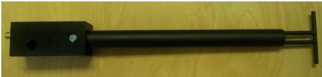
Figure 1 – MVG COMOSAR Validation Dipole
