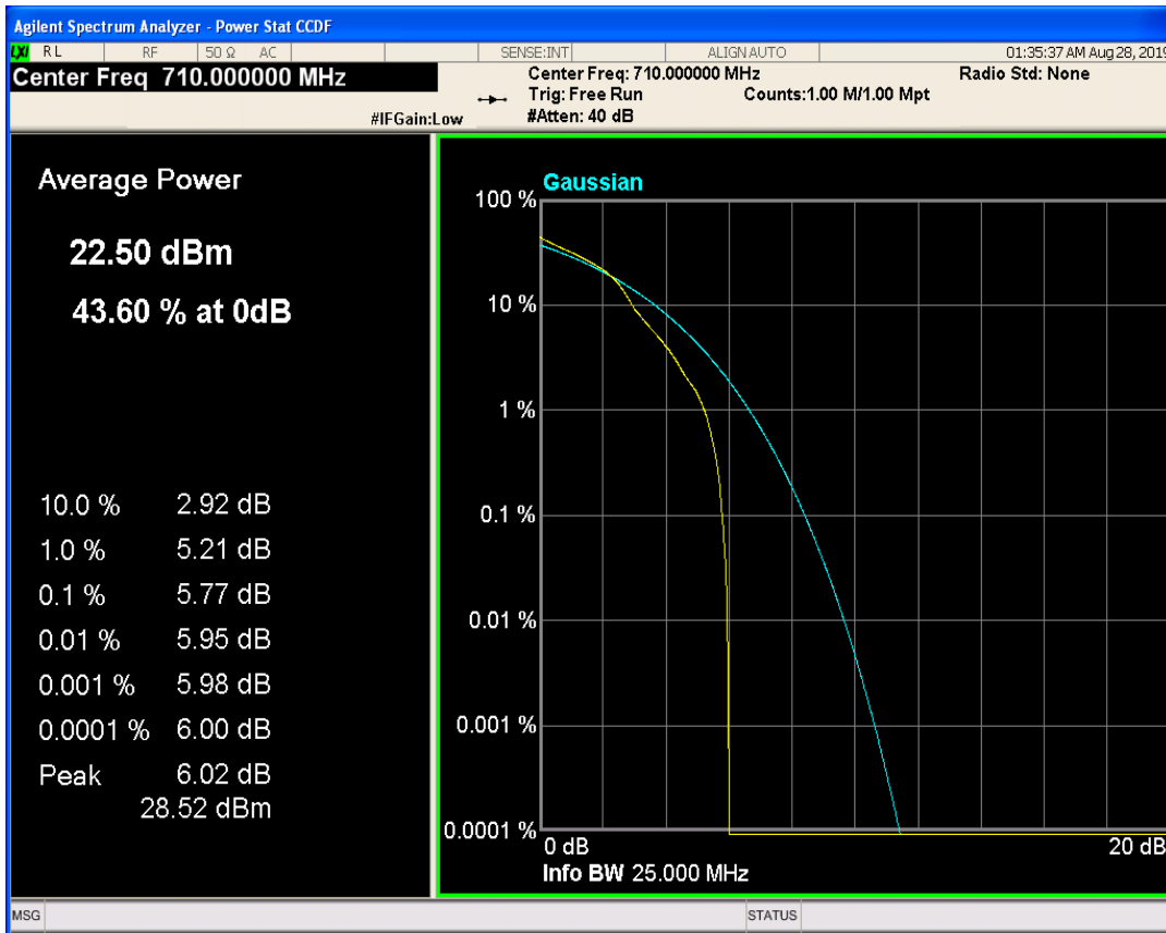
LTE Band2 QPSK BW=1.4MHz Channel=18900 RB Size=1 Position=#0
