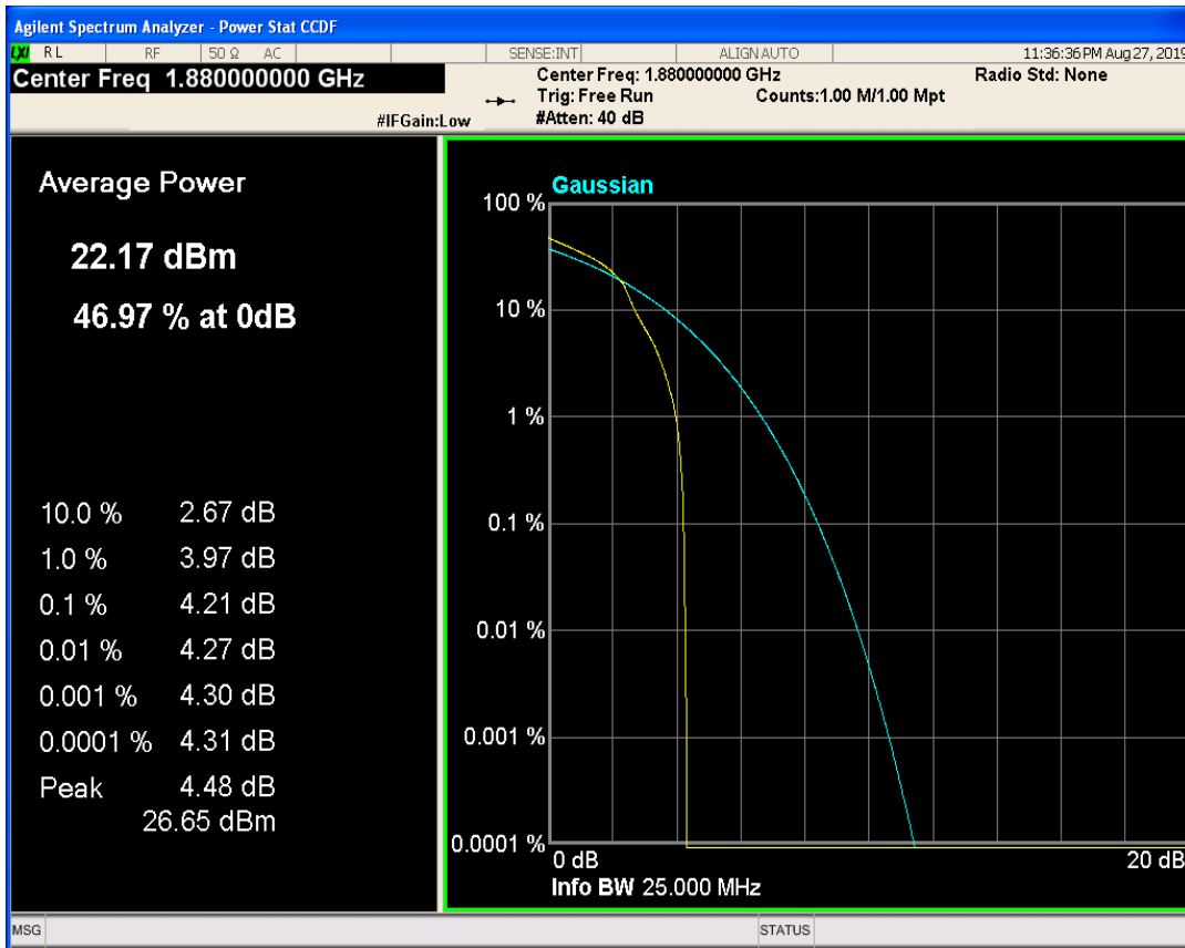
LTE Band4 QPSK BW=1.4MHz Channel=20175 RB Size=1 Position=#0
