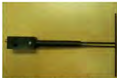
Figure 1 – MVG COMOSAR Validation Dipole
