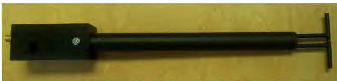
Figure 1 – MVG COMOSAR Validation Dipole
