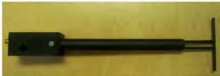
Figure 1 – MVG COMOSAR Validation Dipole
