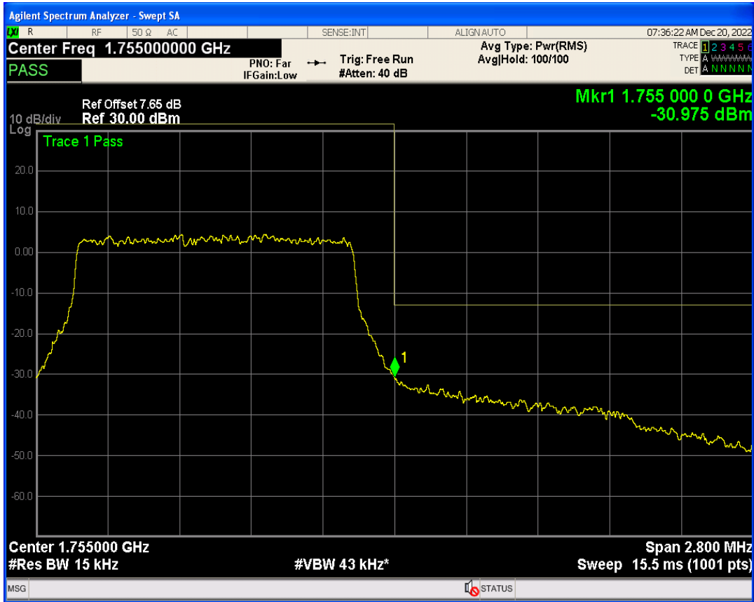
Band4 QPSK BW=3MHz Channel=19965 RB Size=1 Position=#Max
