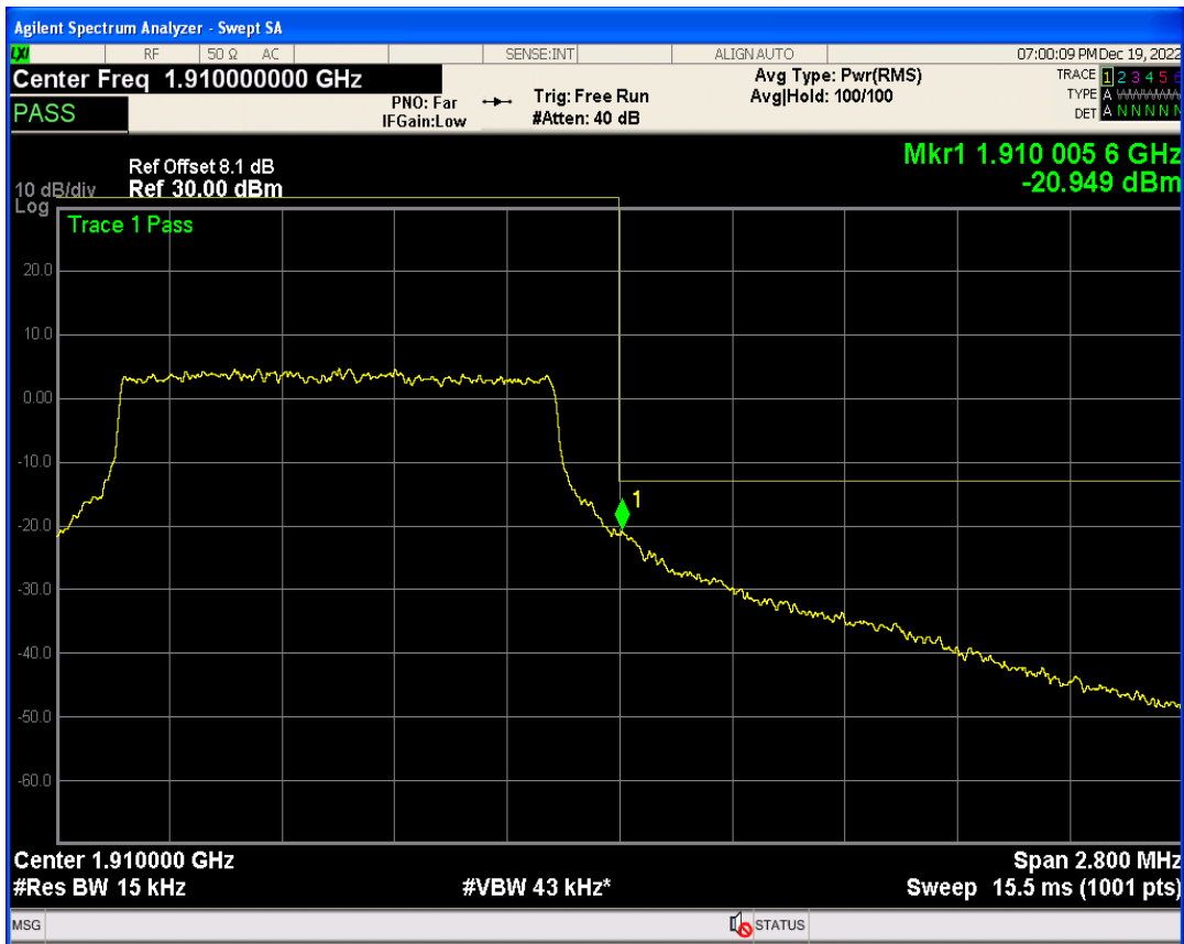
Band2 QPSK BW=3MHz Channel=18615 RB Size=1 Position=#Max
