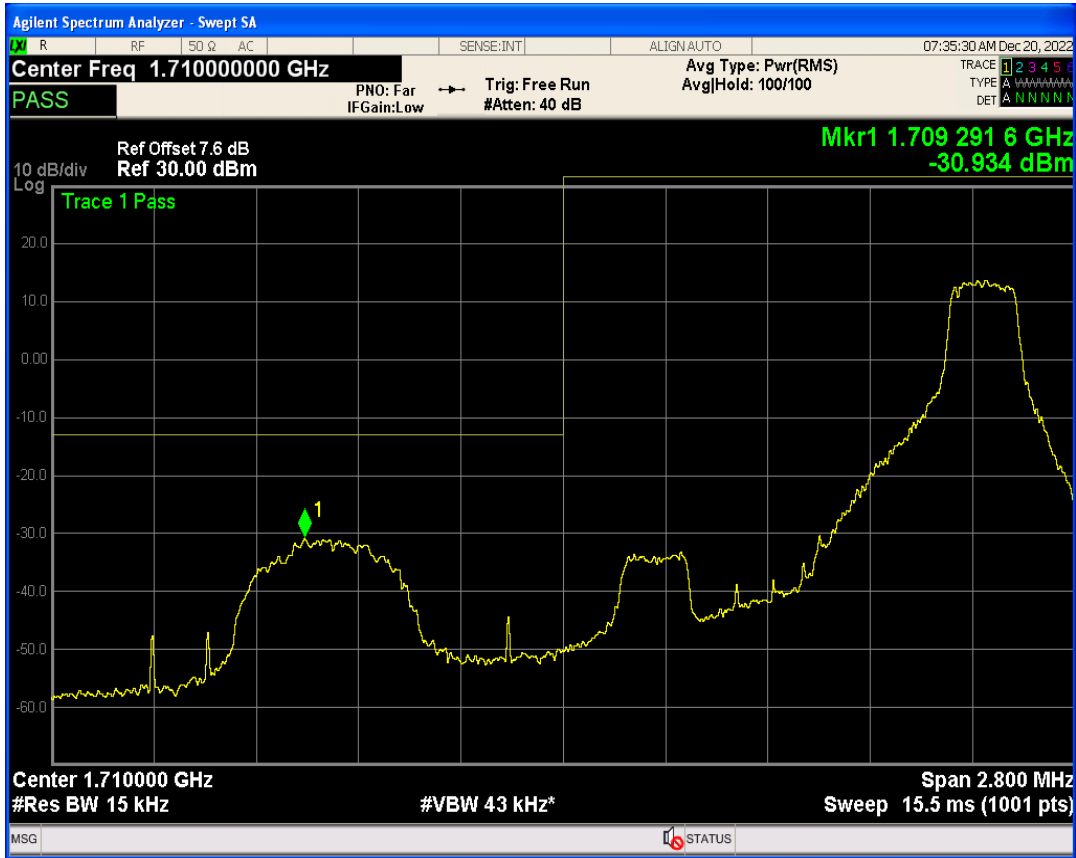
Band4 QPSK BW=1.4MHz Channel=19957 RB Size=6 Position=#0
