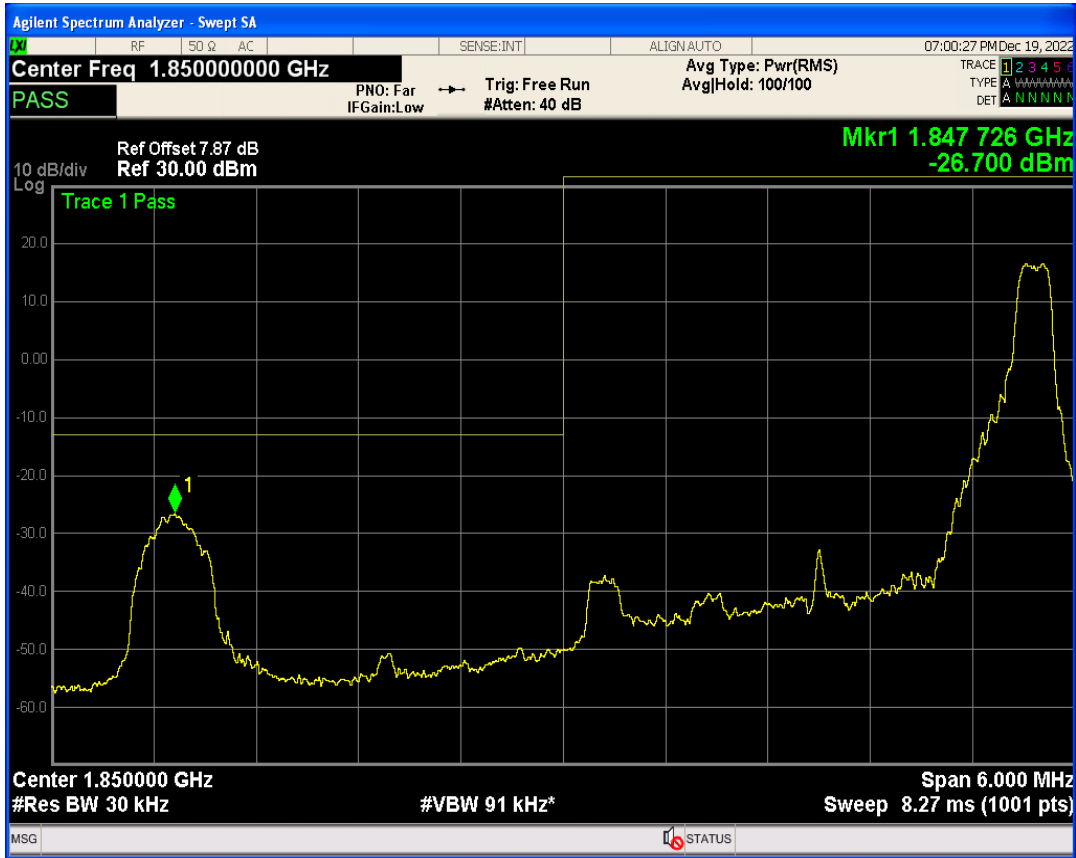
Band2 QAM16 BW=3MHz Channel=18615 RB Size=1 Position=#0
