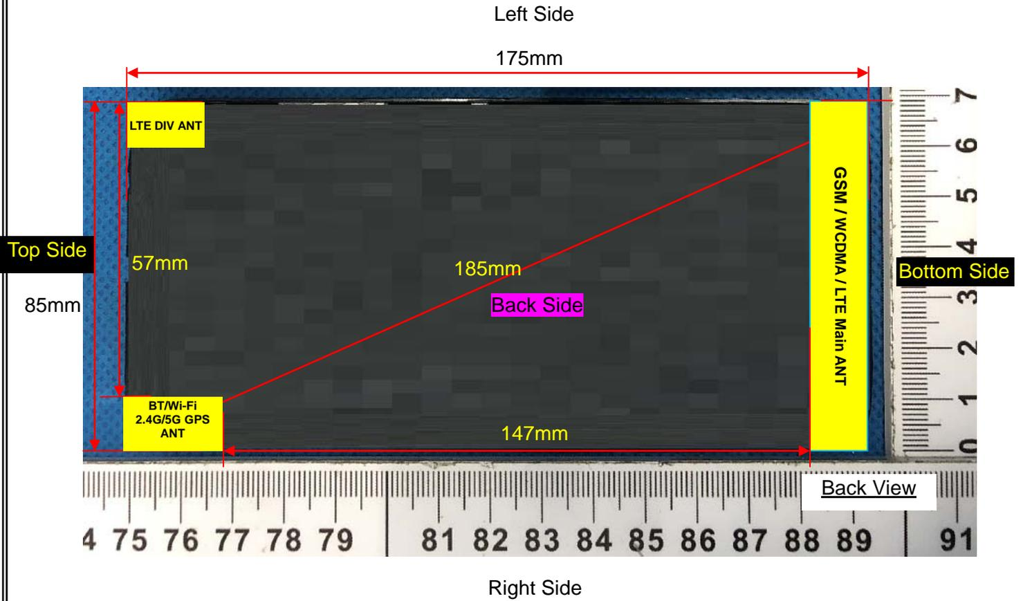
Note: Since the confidentiality request of EUT, the antenna location example diagram see as above.
