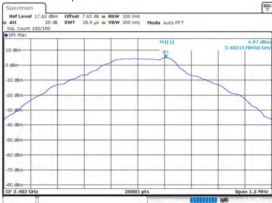
Tx. Spurious NVNT 1-DH5 2402MHz Ant1 Ref
