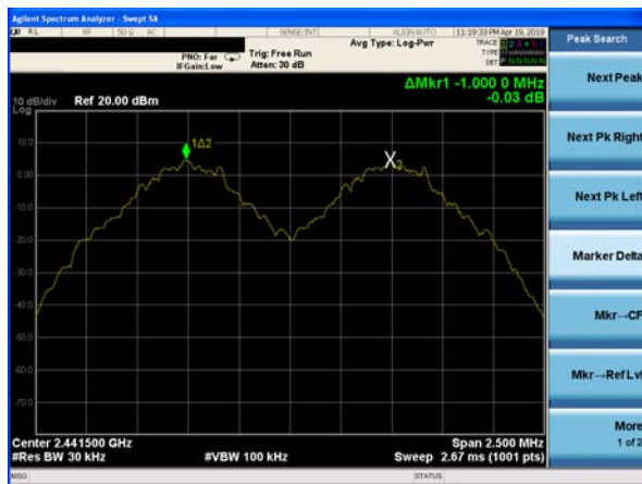
(1Mbps) Channel Separation plot on channel 39-40
