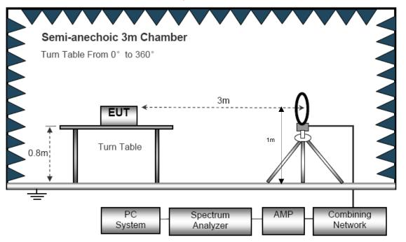
(B) Radiated Emission Test-Up Frequency 30MHz~1GHz
