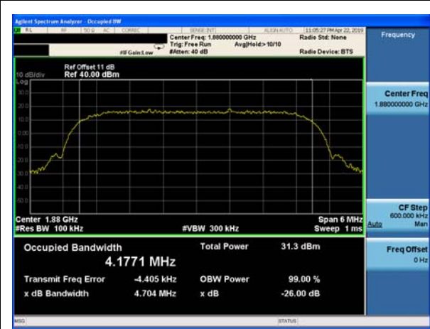
-26dB&99% Bandwidth plot on channel 9400
