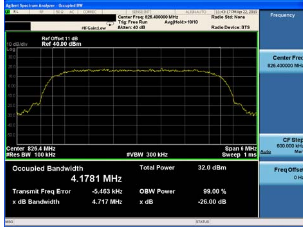
-26dB&99% Bandwidth plot on channel 4183
