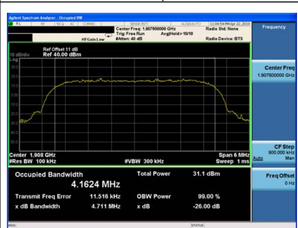
-26dB&99% Bandwidth plot on channel 9538
