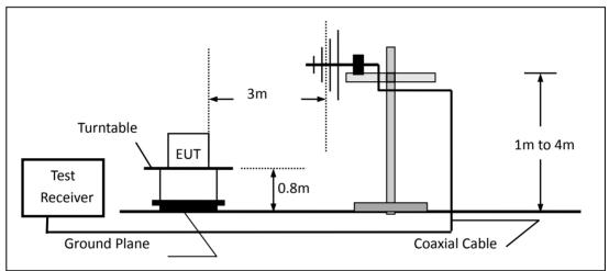
(c) For radiated emissions above 1000MHz
