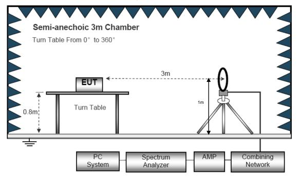
(B) Radiated Emission Test-Up Frequency 30MHz~1GHz
