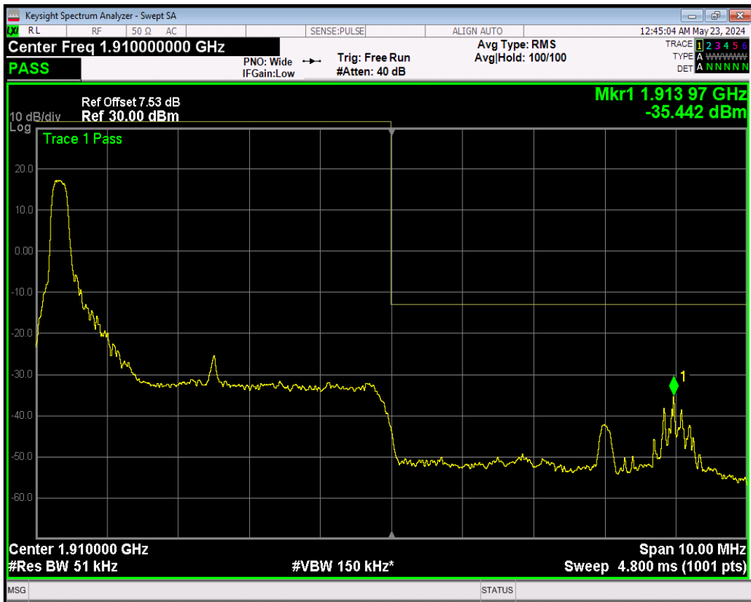
Band2 16QAM BW=5MHz Channel=18625 RB Size=25 Position=#0
