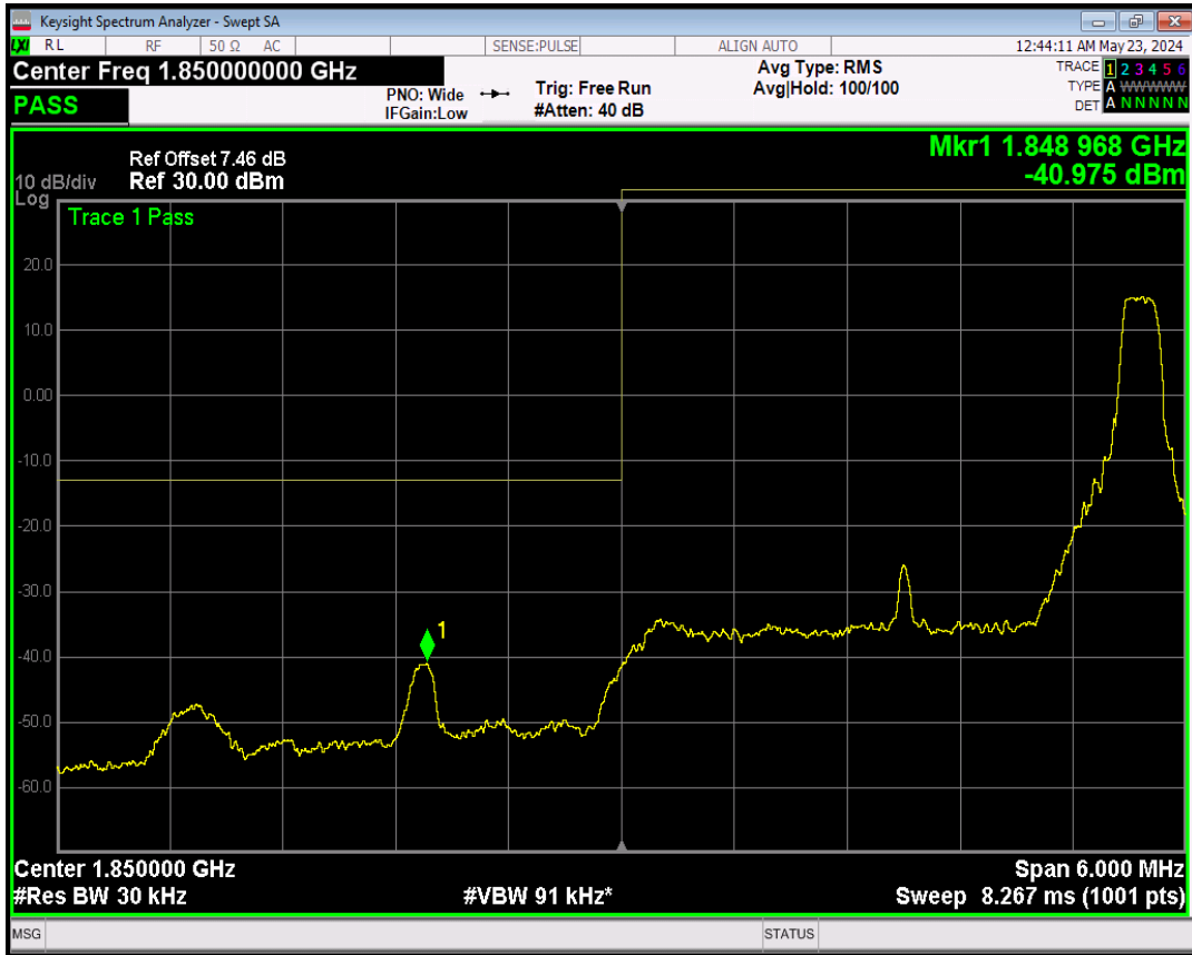
Band2 QPSK BW=20MHz Channel=19100 RB Size=1 Position=#Max
