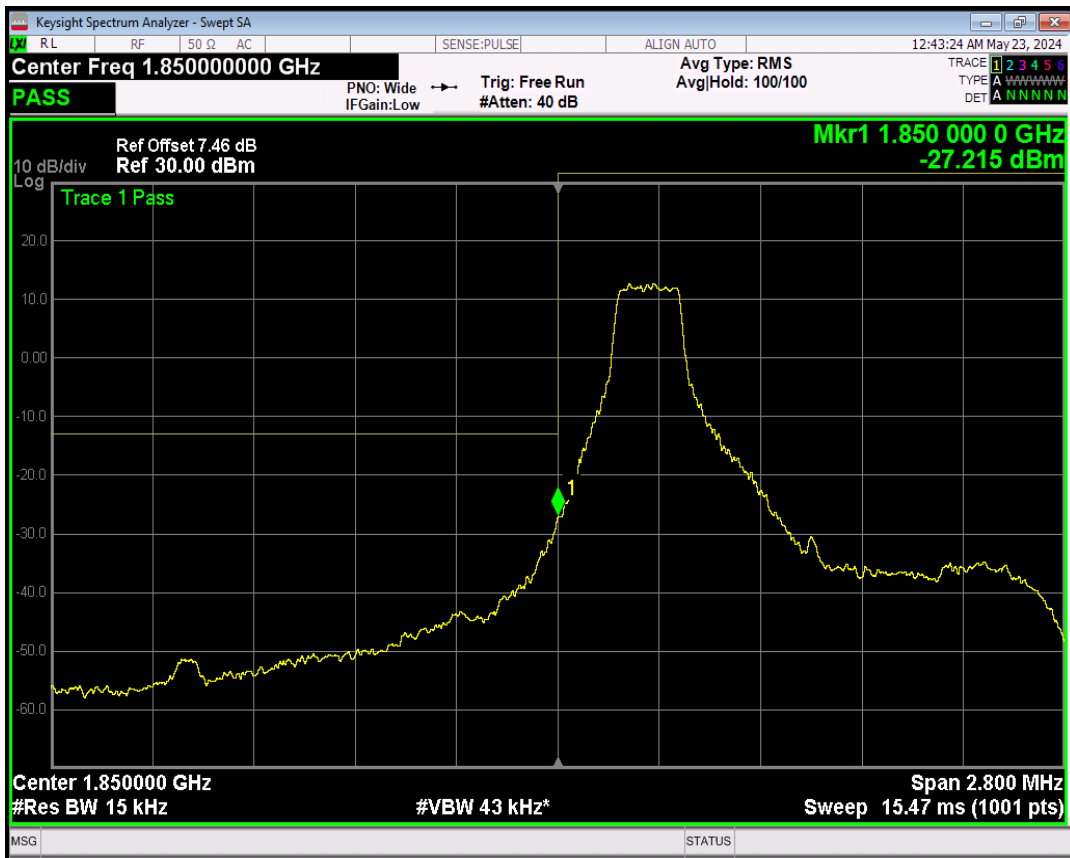
Band2 QPSK BW=1.4MHz Channel=19193 RB Size=6 Position=#0
