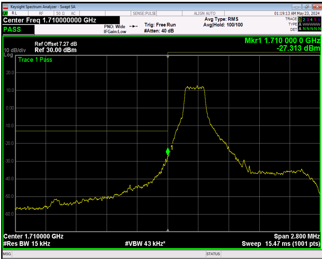
Band4 16QAM BW=1.4MHz Channel=20393 RB Size=1 Position=#0
