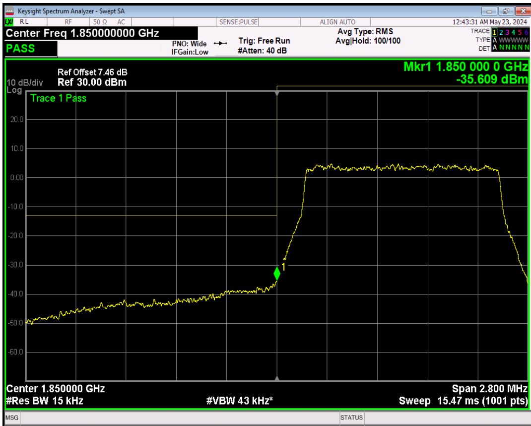
Band2 QPSK BW=1.4MHz Channel=18607 RB Size=1 Position=#Max
