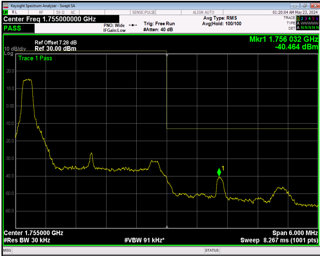
Band4 QPSK BW=3MHz Channel=20385 RB Size=1 Position=#Max
