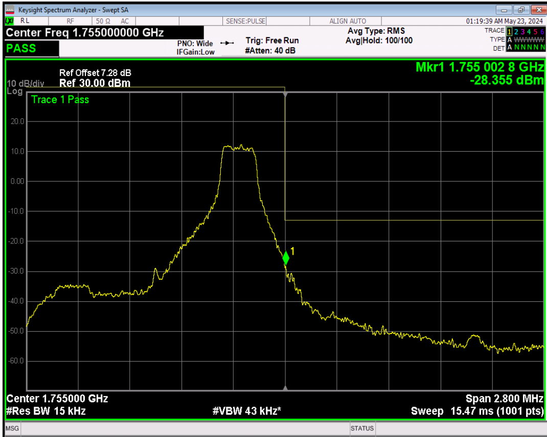
Band4 16QAM BW=10MHz Channel=20000 RB Size=1 Position=#0
