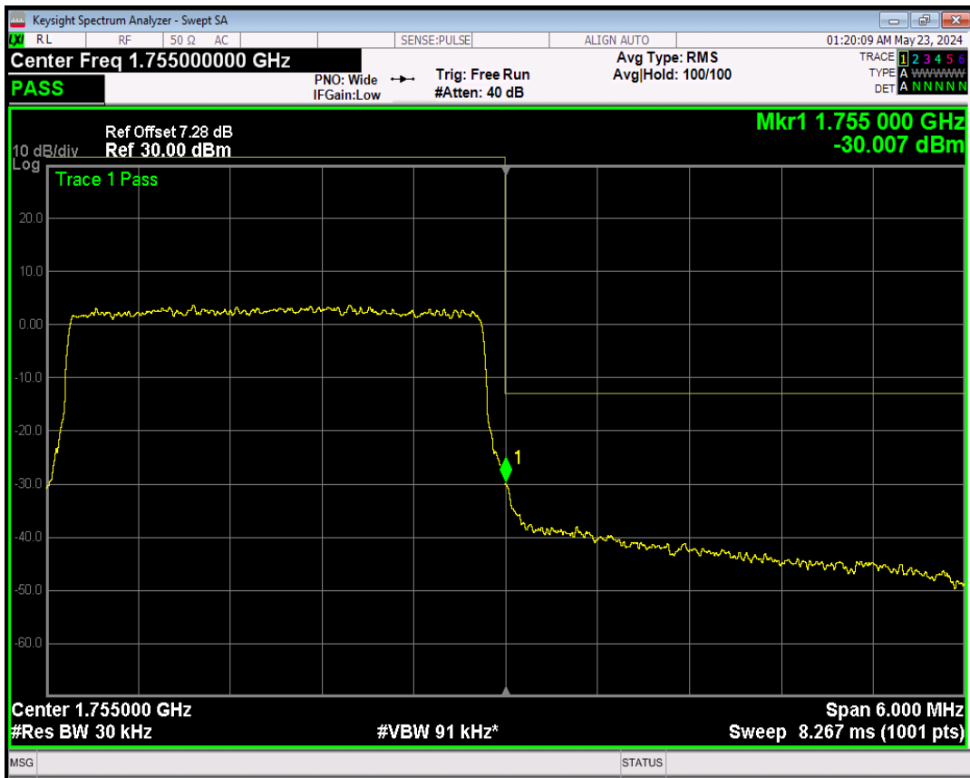
Band4 QPSK BW=5MHz Channel=19975 RB Size=1 Position=#0
