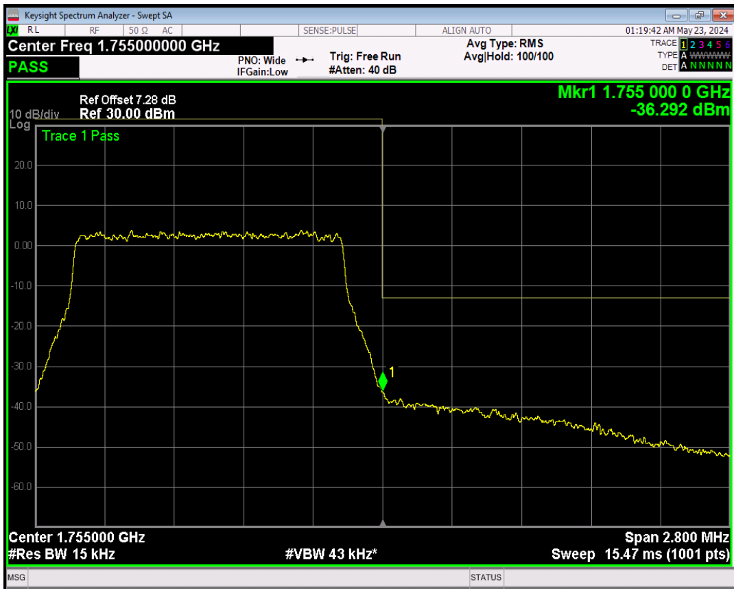
Band4 16QAM BW=1.4MHz Channel=20393 RB Size=1 Position=#Max
