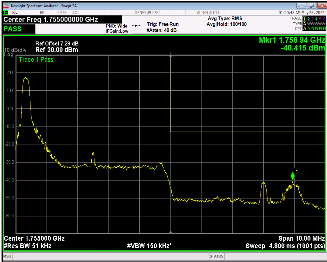
Band4 16QAM BW=5MHz Channel=20375 RB Size=1 Position=#Max
