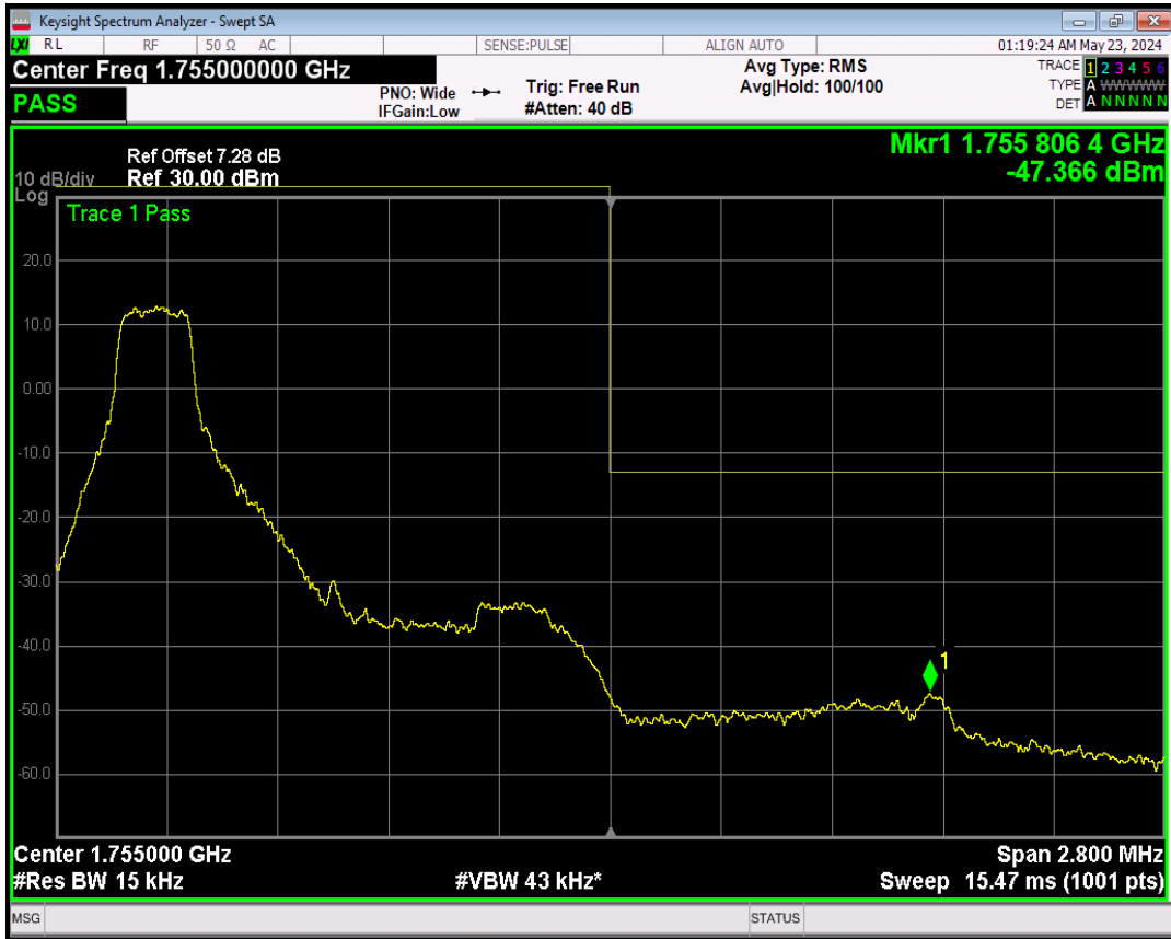
Band4 QPSK BW=1.4MHz Channel=20393 RB Size=1 Position=#Max
