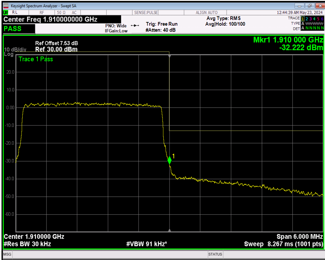
Band2 16QAM BW=5MHz Channel=18625 RB Size=1 Position=#Max
