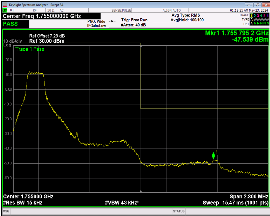
Band4 16QAM BW=1.4MHz Channel=19957 RB Size=6 Position=#0
