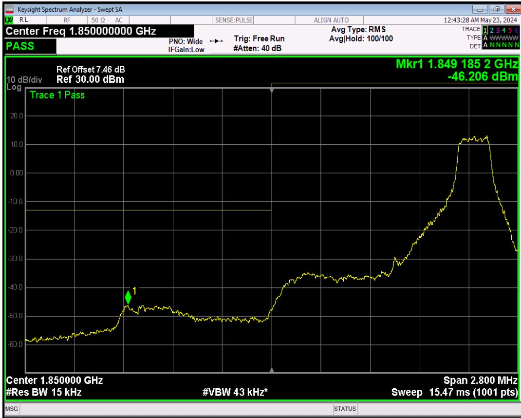
Band2 QPSK BW=1.4MHz Channel=18607 RB Size=1 Position=#0
