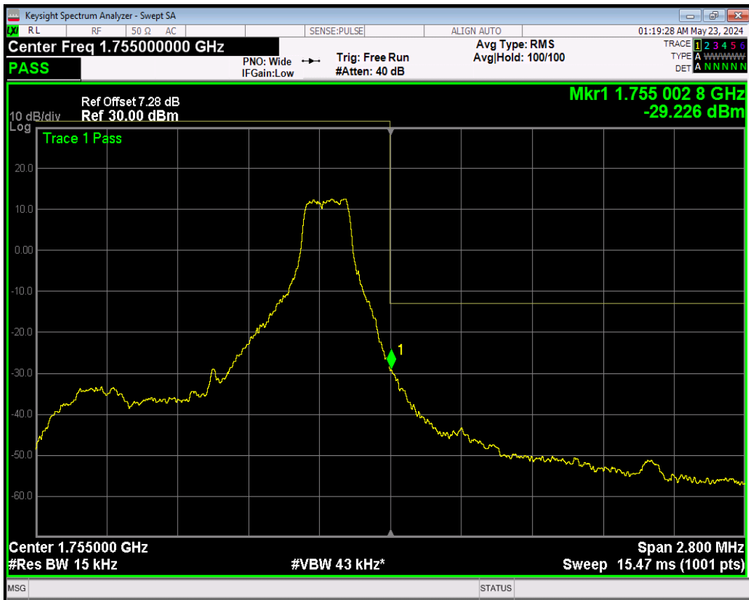
Band4 QPSK BW=10MHz Channel=20000 RB Size=50 Position=#0
