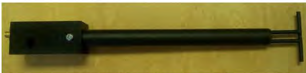
Figure 1 – MVG COMOSAR Validation Dipole
