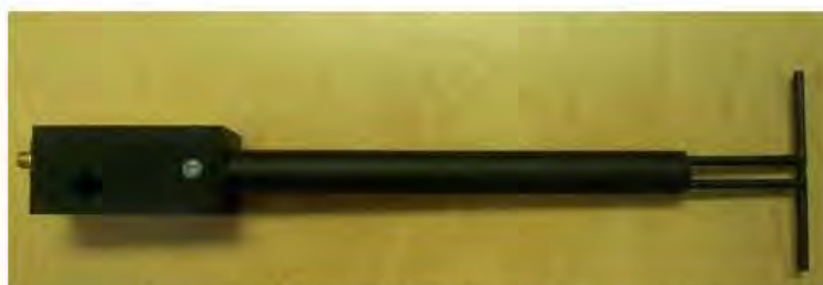
Figure 1 – MVG COMOSAR Validation Dipole
