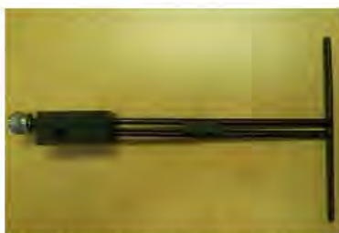
Figure 1 – MVG COMOSAR Validation Dipole
