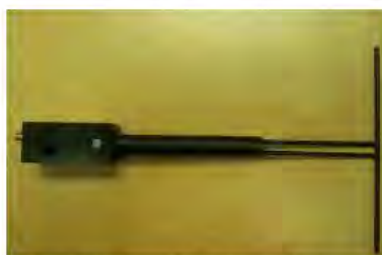
Figure 1 – MVG COMOSAR Validation Dipole
