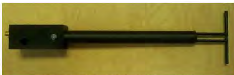
Figure 1 – MVG COMOSAR Validation Dipole
