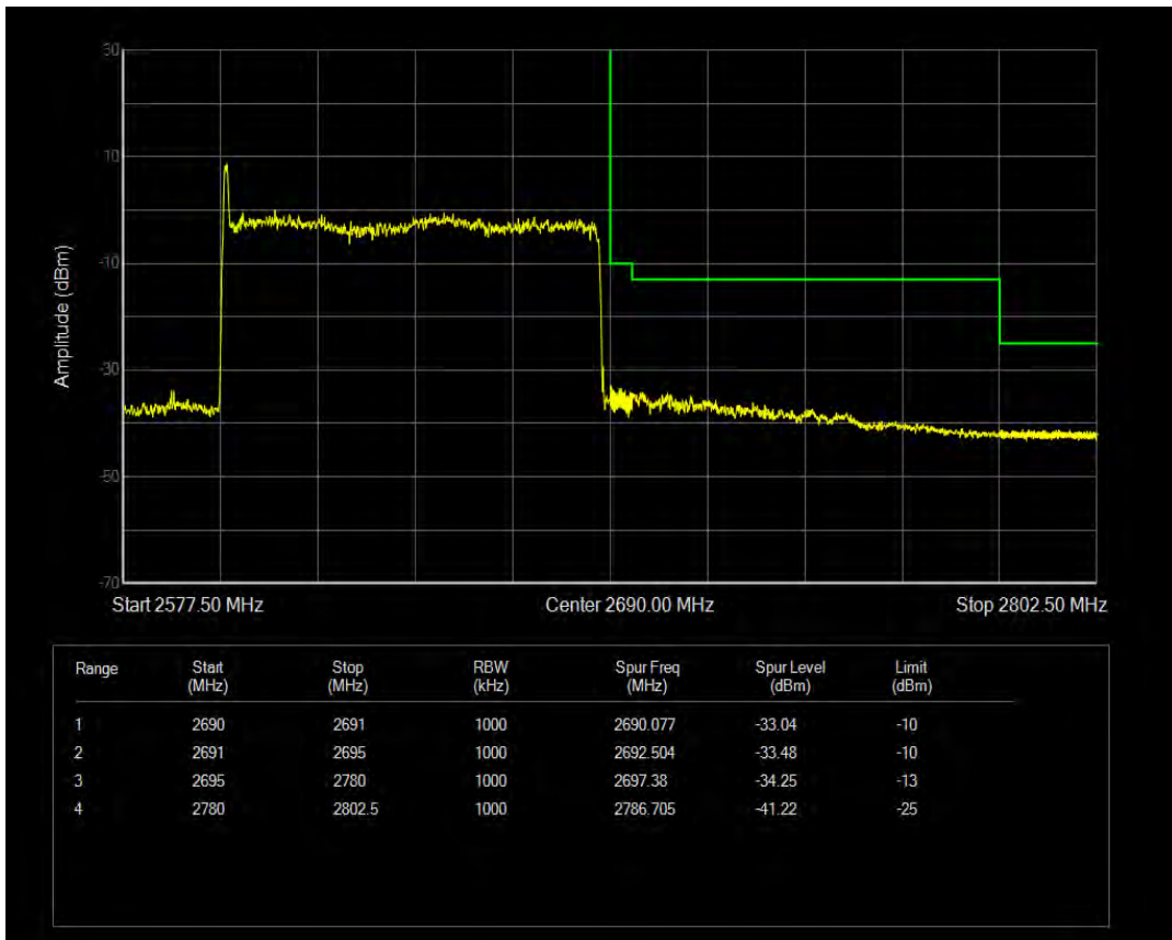
n78 SCS=30kHz DFT_QPSK BW=100MHz Channel=633333 RB=1@0
