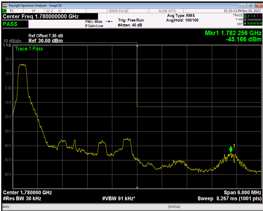
Band66 QPSK BW=3MHz Channel=132657 RB Size=1 Position=#Max
