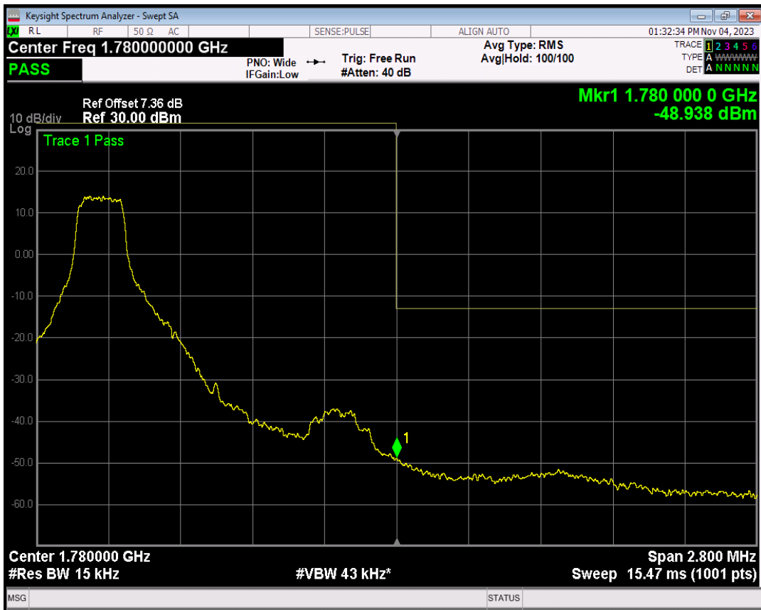
Band66 QPSK BW=1.4MHz Channel=132665 RB Size=1 Position=#Max
