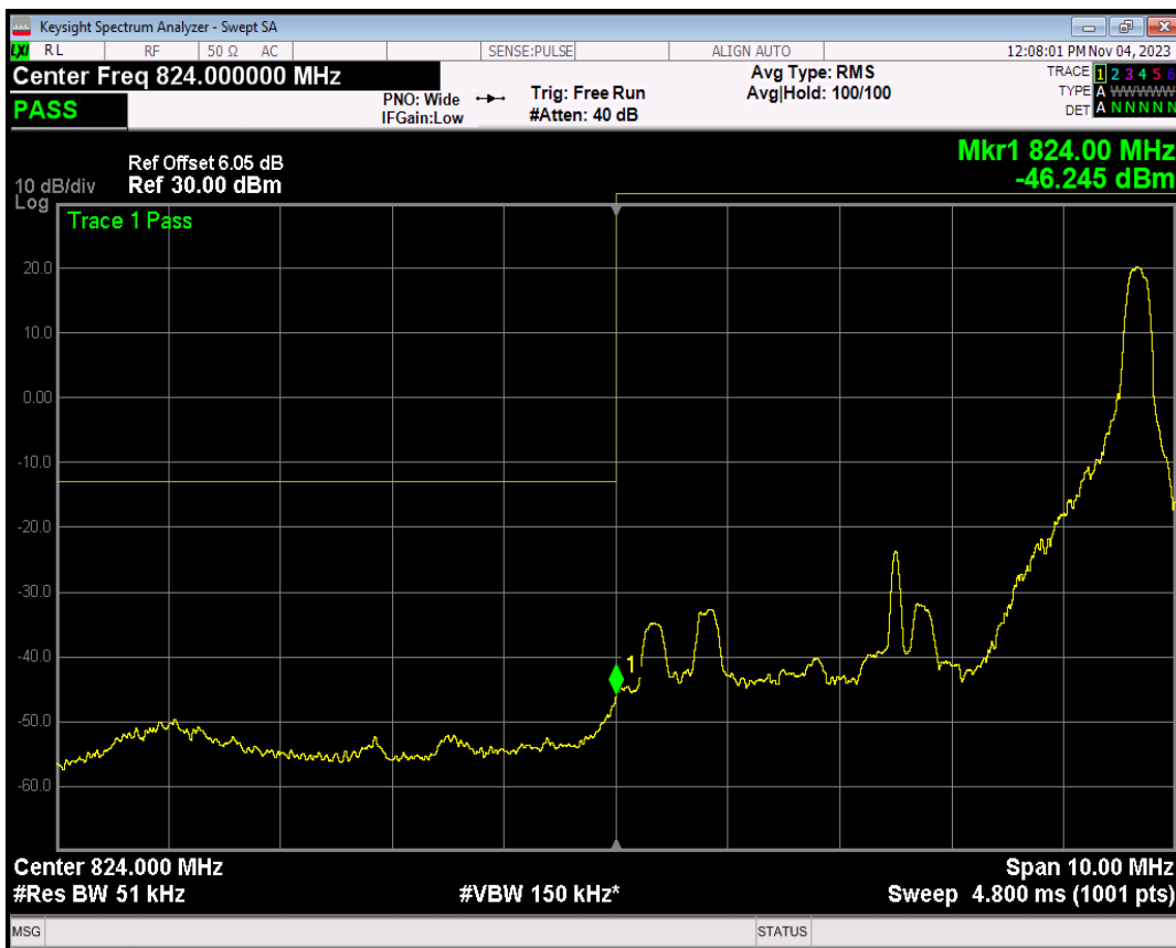
Band5 QPSK BW=5MHz Channel=20425 RB Size=25 Position=#0
