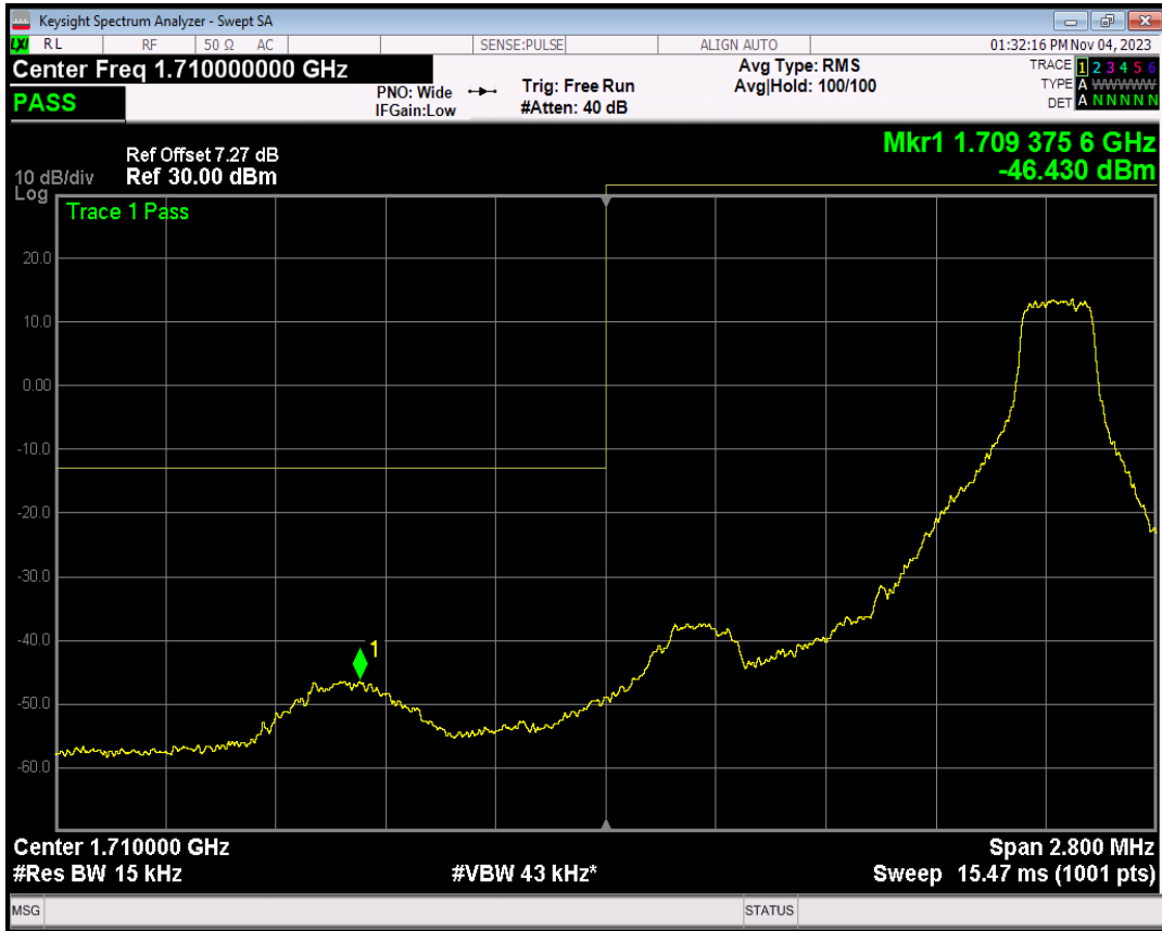
Band66 16QAM BW=1.4MHz Channel=131979 RB Size=1 Position=#0
