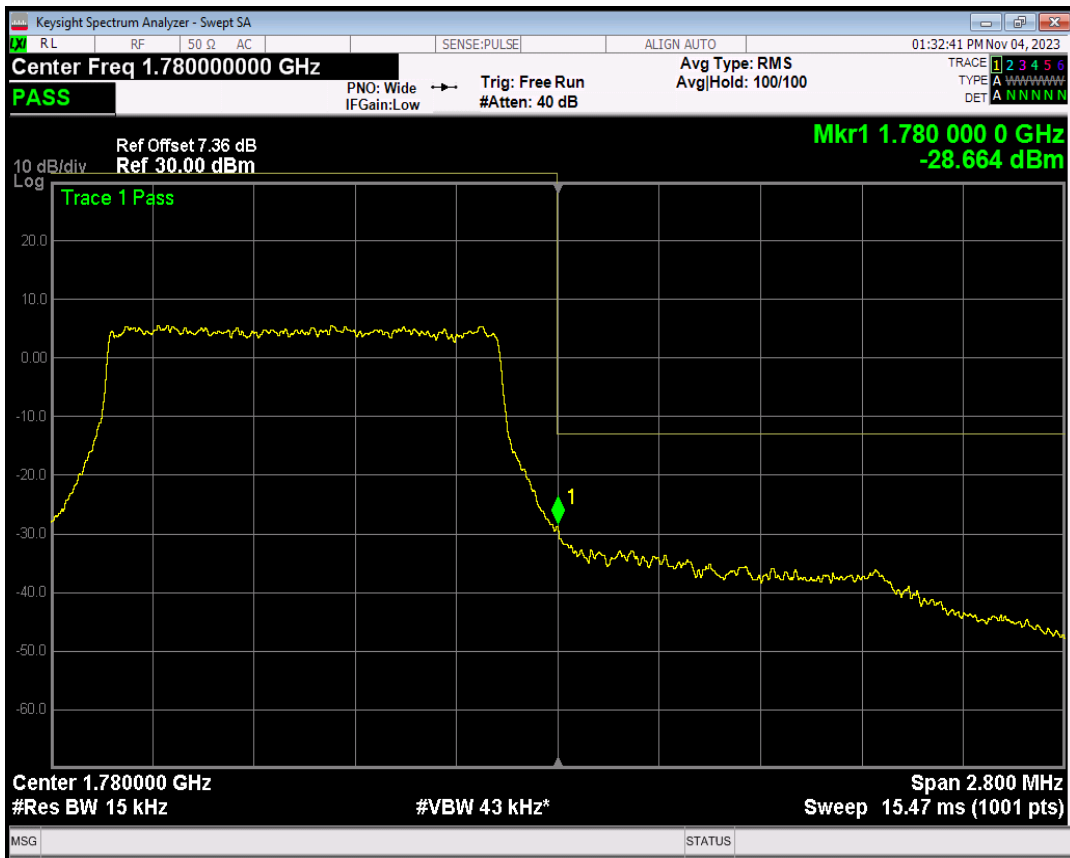
Band66 16QAM BW=1.4MHz Channel=132665 RB Size=1 Position=#0
