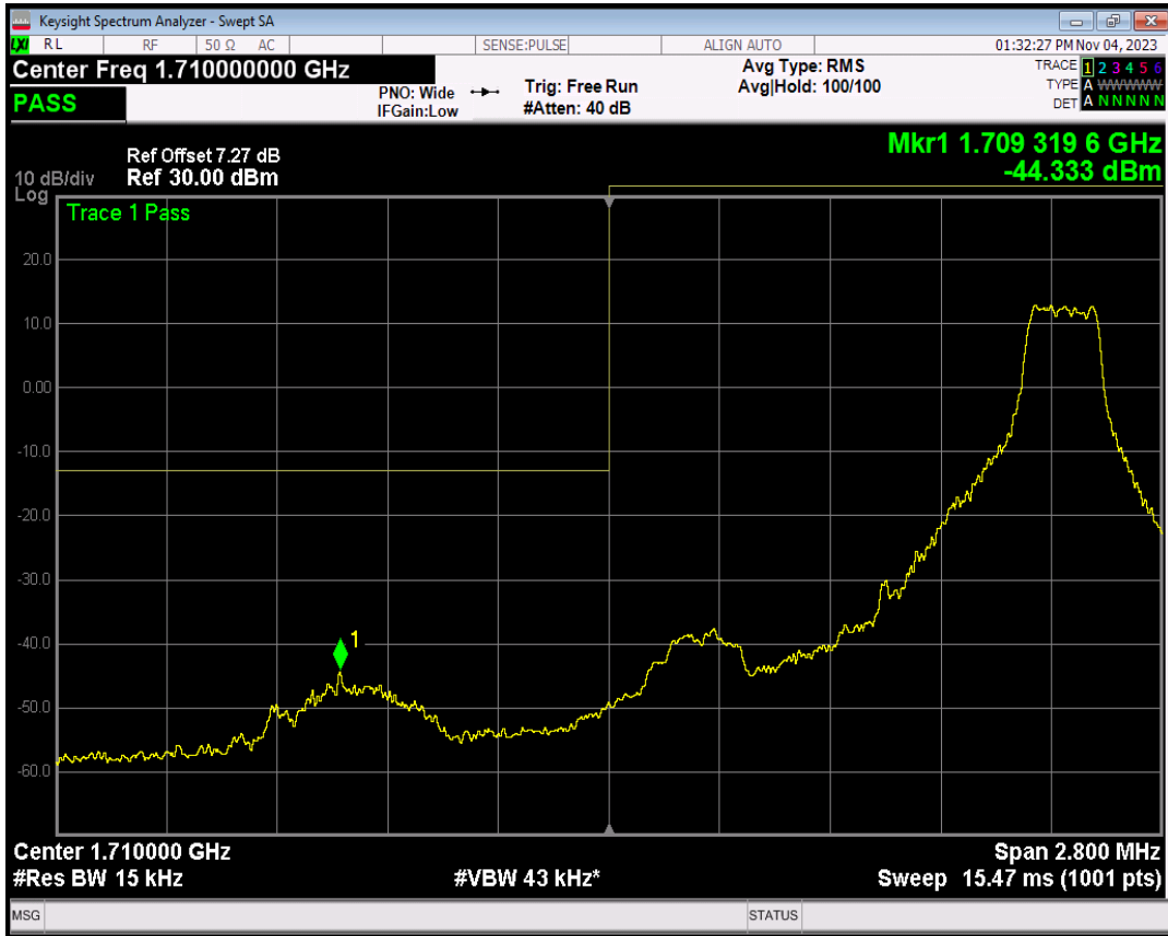
Band66 QPSK BW=1.4MHz Channel=132665 RB Size=1 Position=#0
