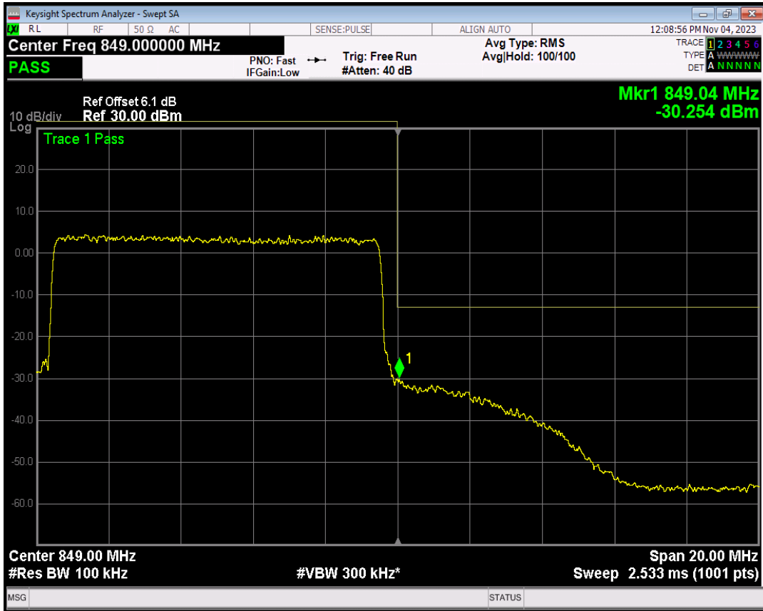
Band66 QPSK BW=1.4MHz Channel=131979 RB Size=1 Position=#0
