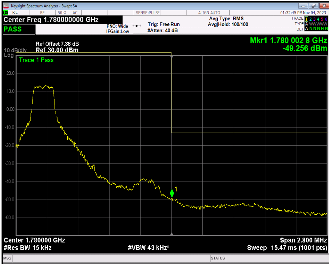
Band66 16QAM BW=1.4MHz Channel=132665 RB Size=1 Position=#Max
