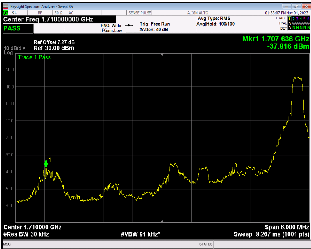
Band66 16QAM BW=3MHz Channel=131987 RB Size=15 Position=#0
