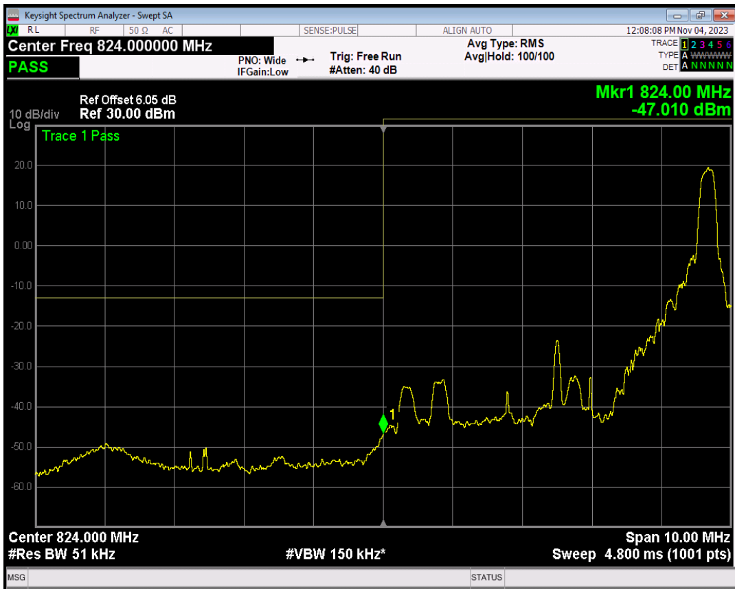
Band5 16QAM BW=5MHz Channel=20425 RB Size=25 Position=#0
