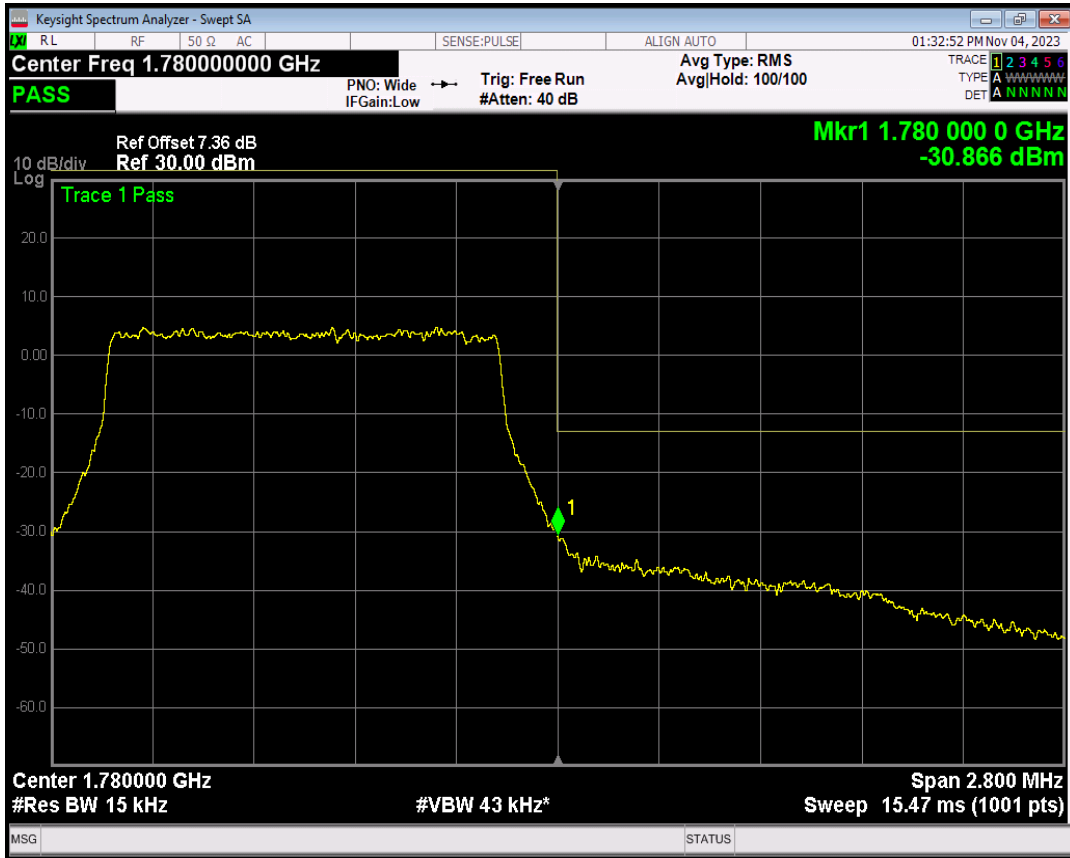
Band66 QPSK BW=3MHz Channel=131987 RB Size=1 Position=#0
