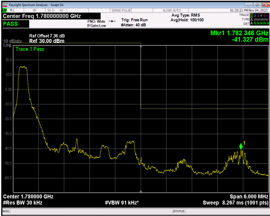
Band66 16QAM BW=3MHz Channel=132657 RB Size=1 Position=#Max
