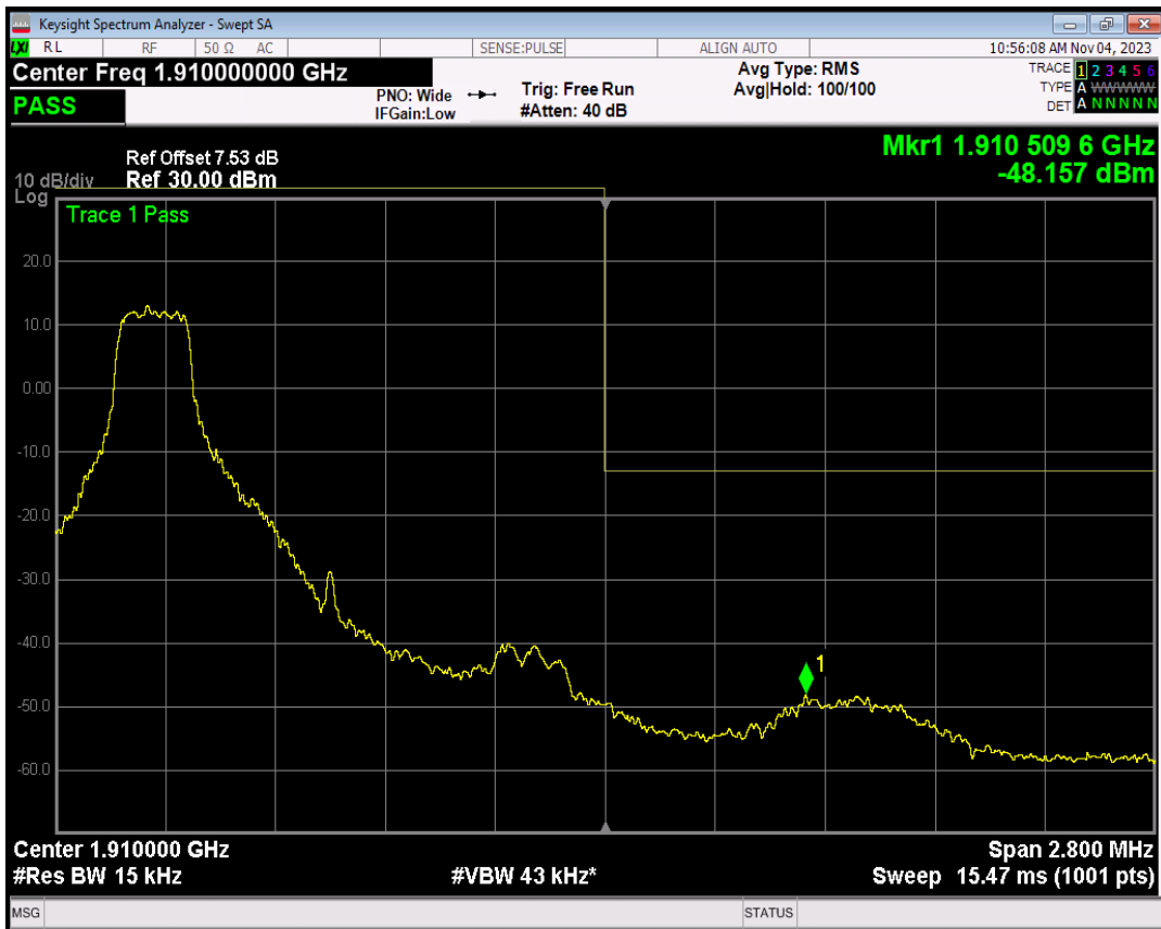
Band2 QPSK BW=1.4MHz Channel=19193 RB Size=1 Position=#Max
