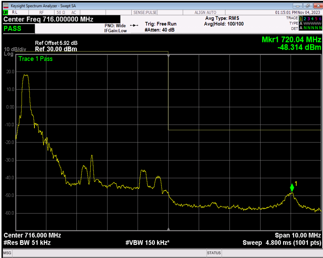
Band17 16QAM BW=5MHz Channel=23825 RB Size=1 Position=#Max
