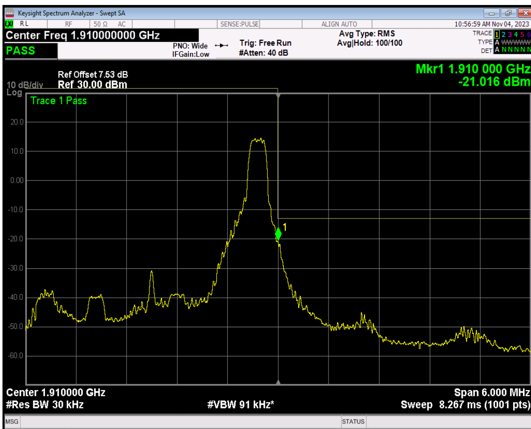
Band2 16QAM BW=3MHz Channel=19185 RB Size=15 Position=#0
