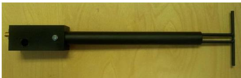
Figure 1 – MVG COMOSAR Validation Dipole
