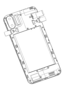
2) Remove the battery, and install SIM and SD cards, place the cards with chip facing downwards, and then slide it into its slot. Make sure that it is correctly inserted.
