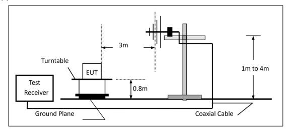
(c) For radiated emissions above 1000MHz
