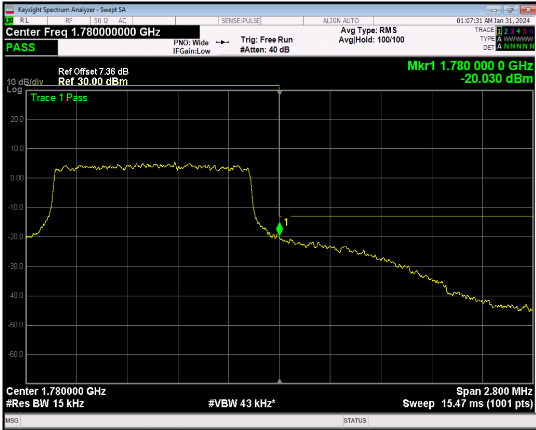
Band66 16QAM BW=1.4MHz Channel=132665 RB Size=1 Position=#0
