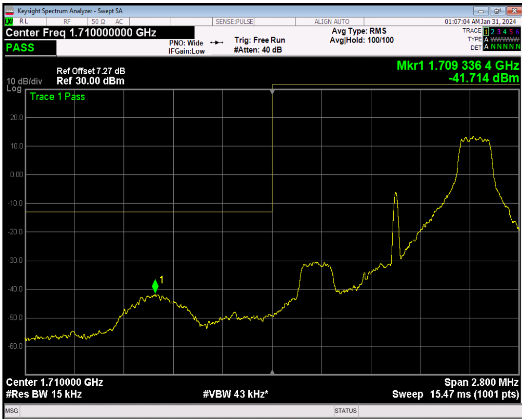
Band66 QPSK BW=1.4MHz Channel=131979 RB Size=6 Position=#0
