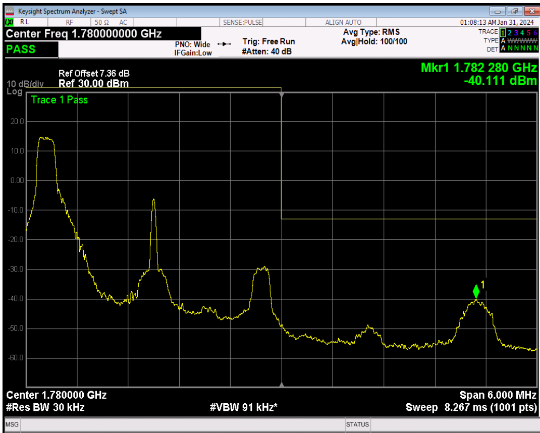
Band66 16QAM BW=3MHz Channel=132657 RB Size=1 Position=#Max
