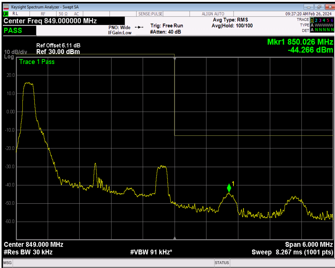
Band5 16QAM BW=3MHz Channel=20635 RB Size=1 Position=#Max
