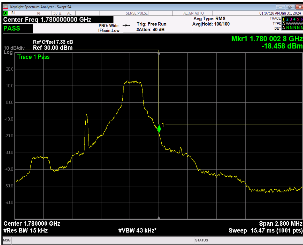
Band66 QPSK BW=1.4MHz Channel=132665 RB Size=6 Position=#0
