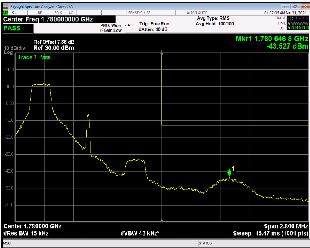
Band66 16QAM BW=1.4MHz Channel=132665 RB Size=1 Position=#Max
