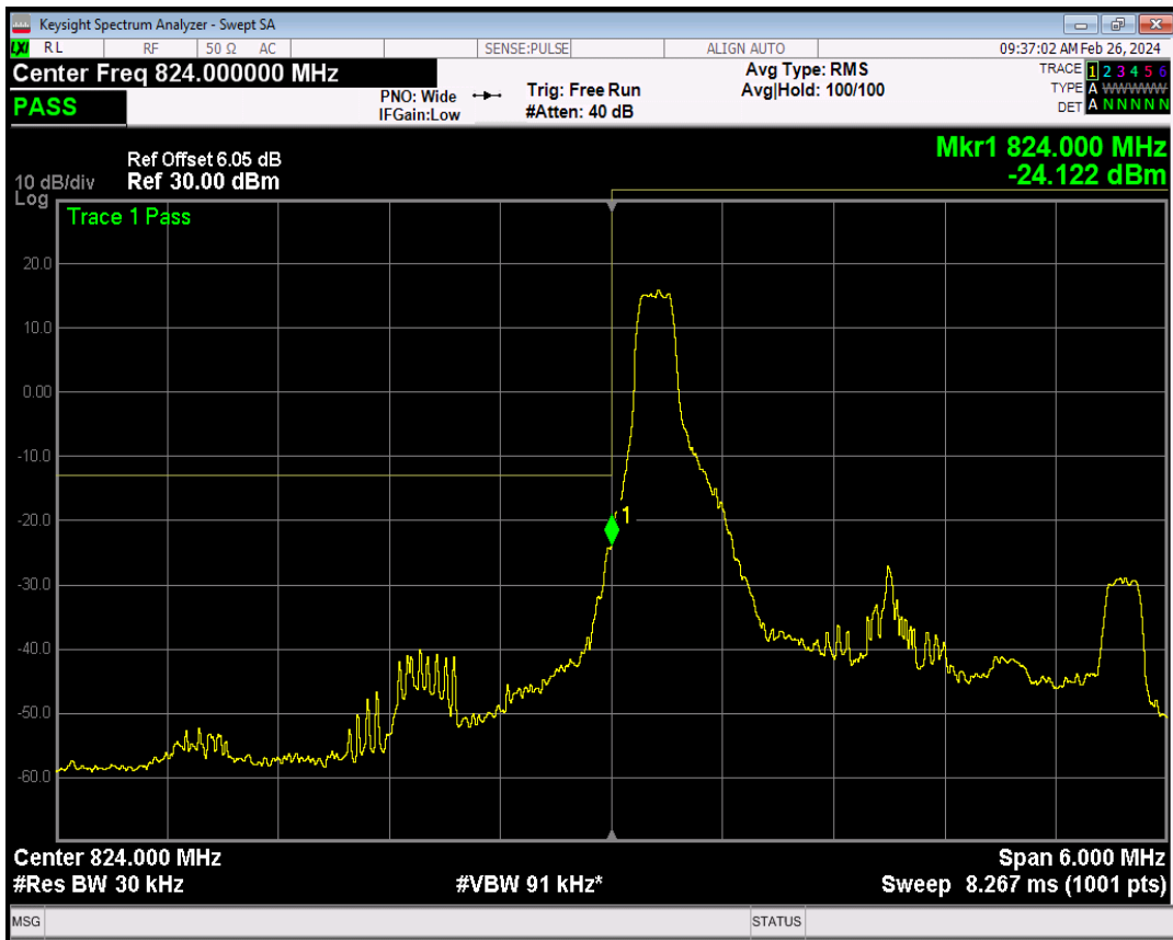
Band5 16QAM BW=3MHz Channel=20415 RB Size=1 Position=#Max
