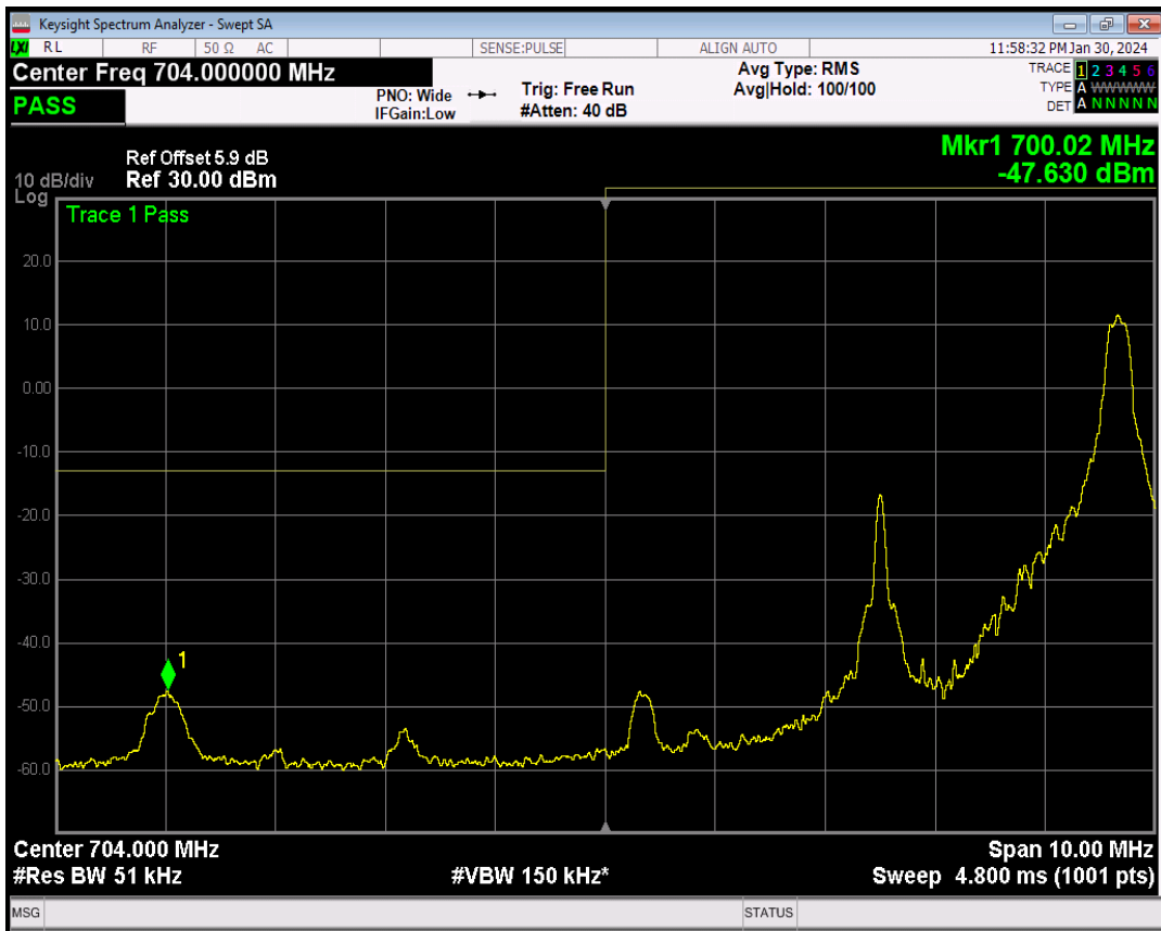
Band17 QPSK BW=5MHz Channel=23755 RB Size=25 Position=#0
