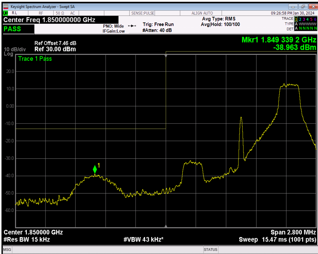
Band2 QPSK BW=1.4MHz Channel=18607 RB Size=6 Position=#0
