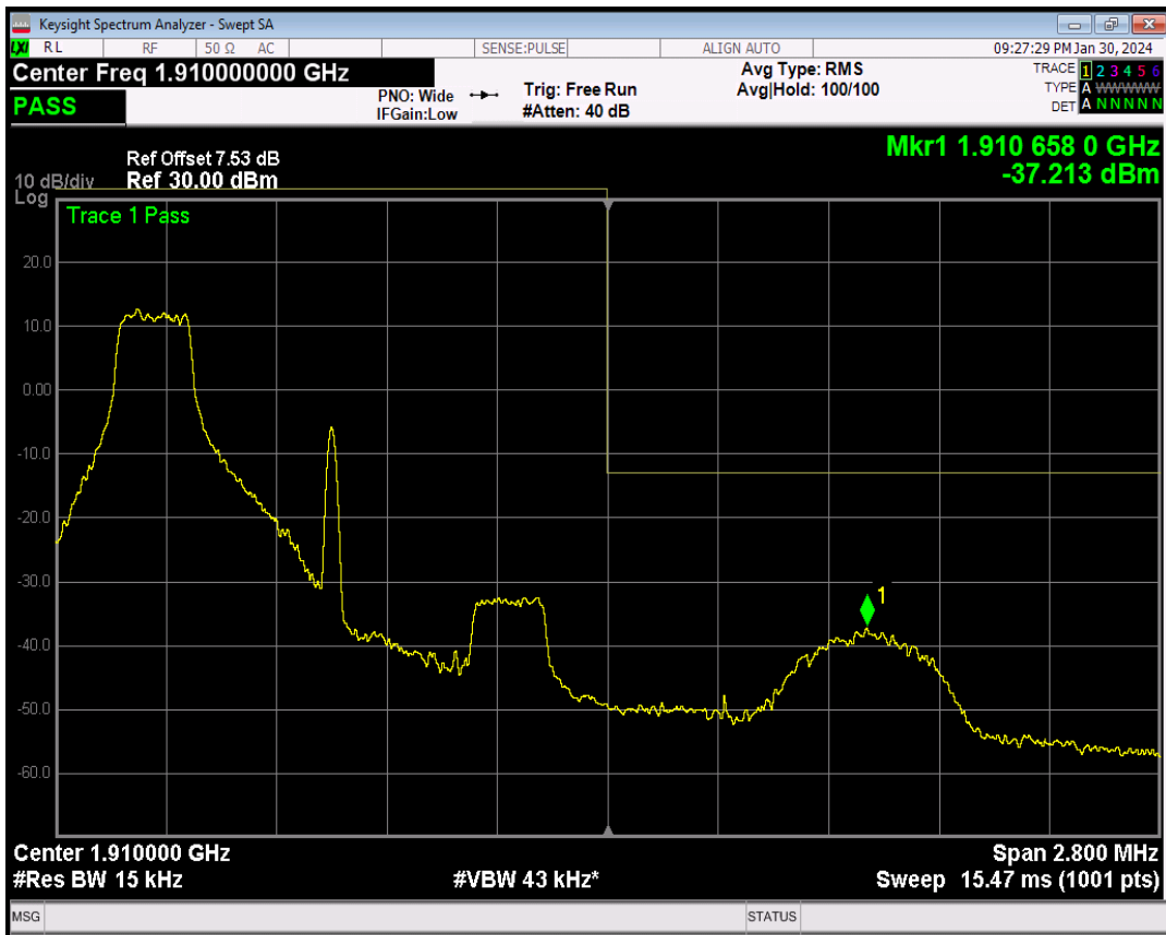
Band2 16QAM BW=1.4MHz Channel=19193 RB Size=1 Position=#Max
