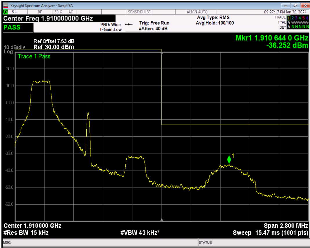
Band2 QPSK BW=1.4MHz Channel=19193 RB Size=1 Position=#Max
