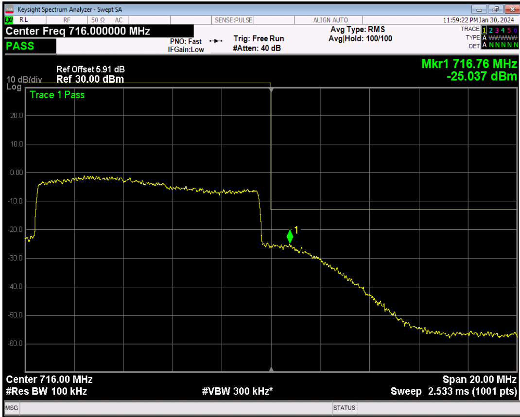
Band17 16QAM BW=10MHz Channel=23800 RB Size=1 Position=#0
