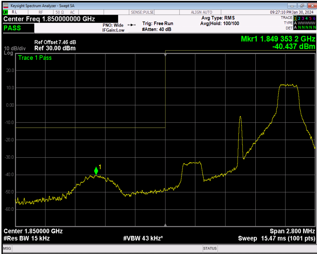
Band2 16QAM BW=1.4MHz Channel=18607 RB Size=6 Position=#0
