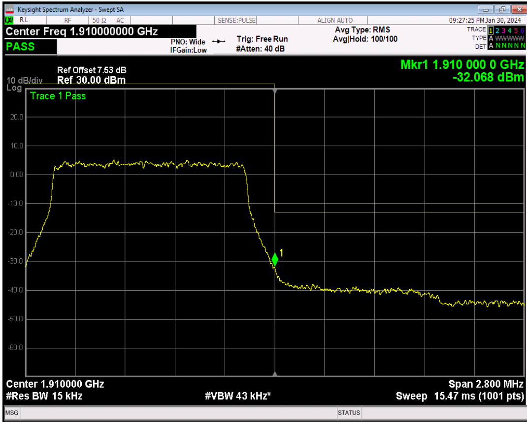
Band2 16QAM BW=1.4MHz Channel=19193 RB Size=1 Position=#0
