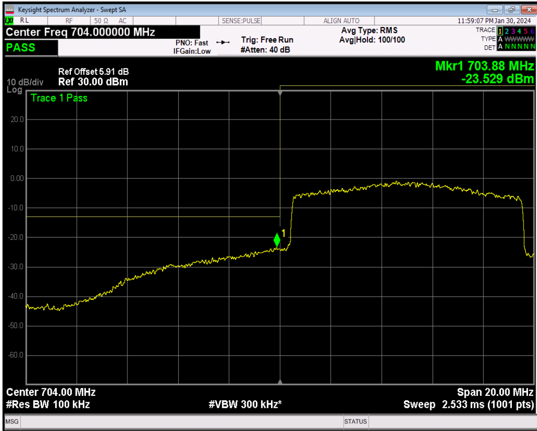
Band17 16QAM BW=10MHz Channel=23780 RB Size=1 Position=#0
