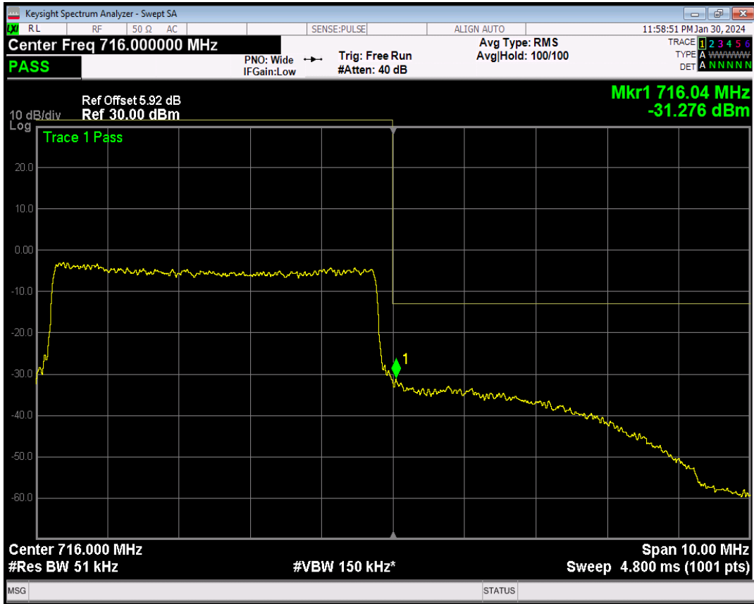
Band17 16QAM BW=5MHz Channel=23825 RB Size=1 Position=#0
