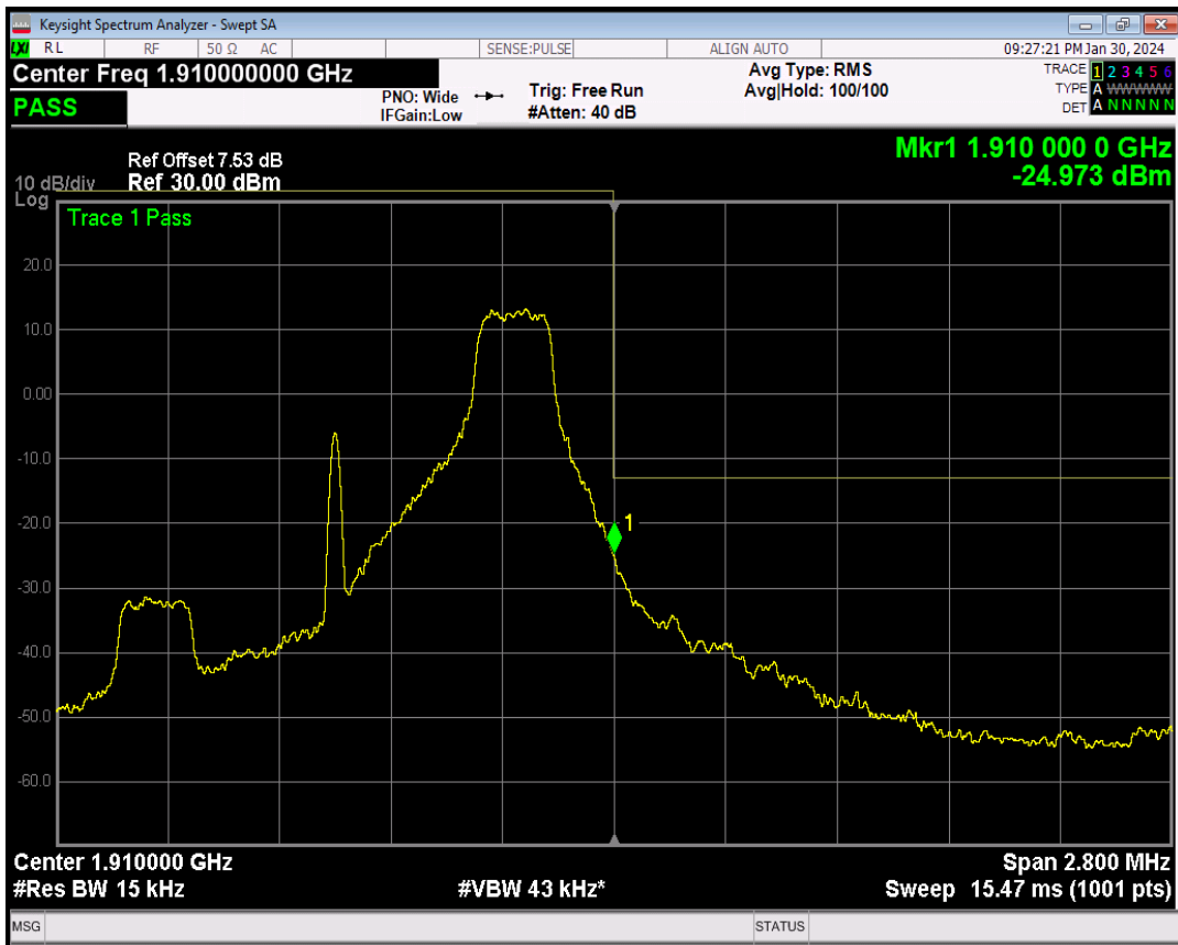
Band2 QPSK BW=1.4MHz Channel=19193 RB Size=6 Position=#0
