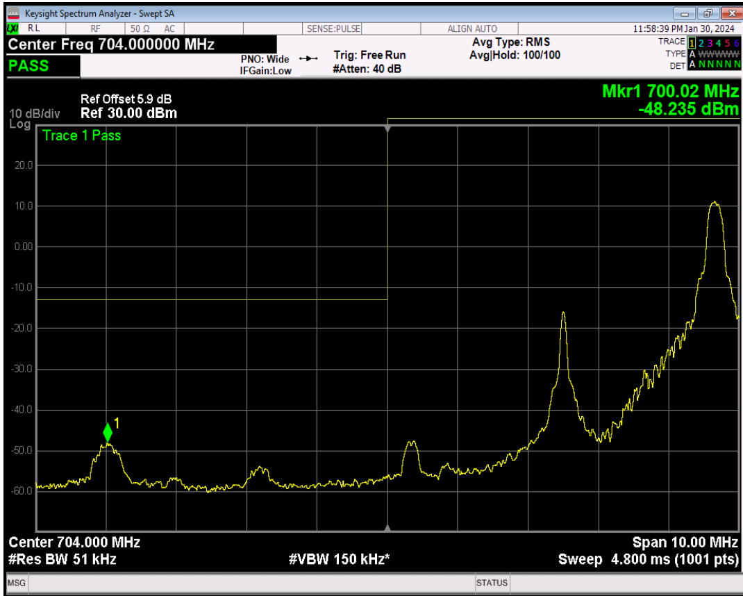
Band17 16QAM BW=5MHz Channel=23755 RB Size=25 Position=#0
