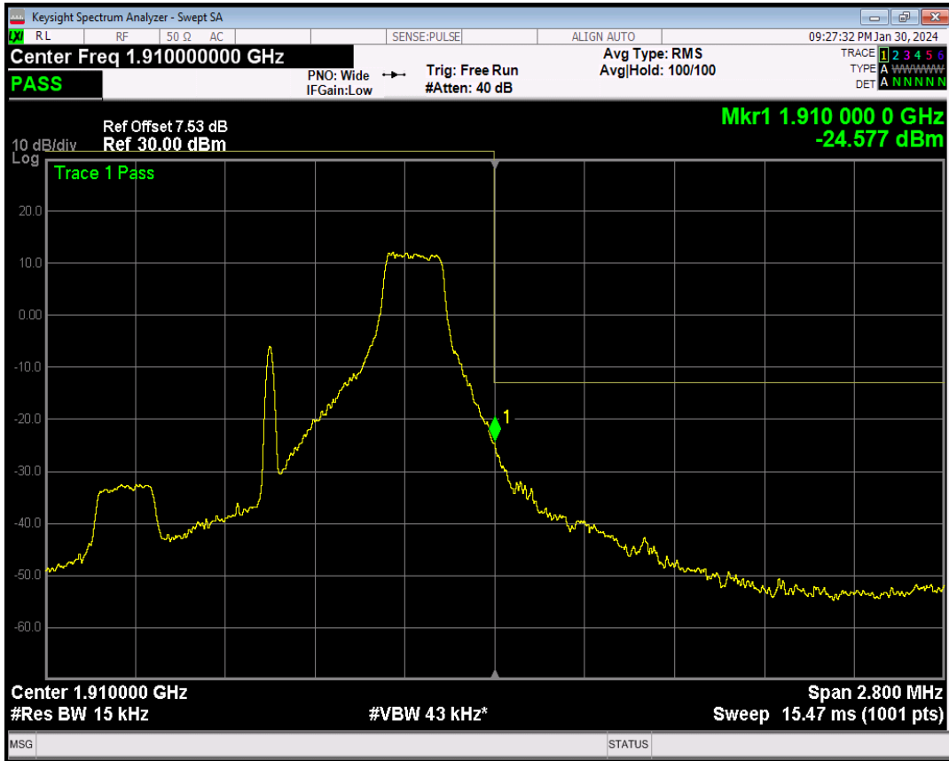
Band2 16QAM BW=1.4MHz Channel=19193 RB Size=6 Position=#0
