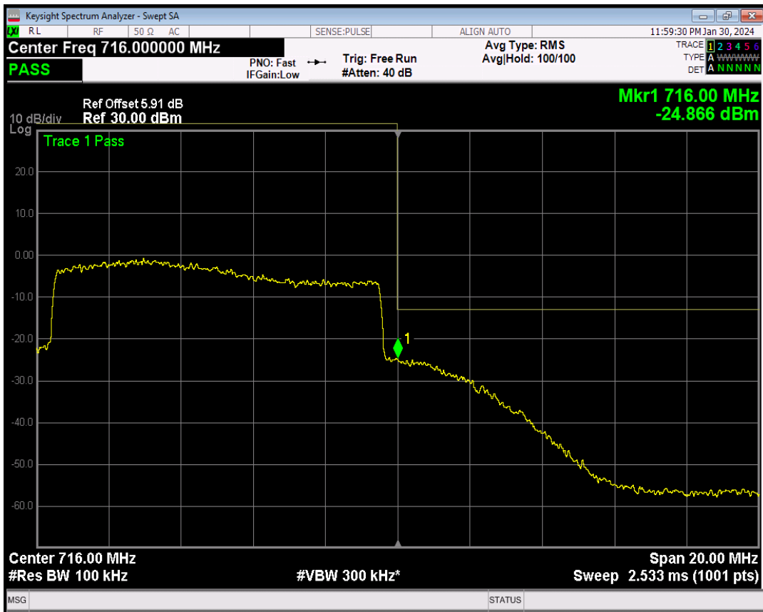
Band2 QPSK BW=1.4MHz Channel=18607 RB Size=1 Position=#0
