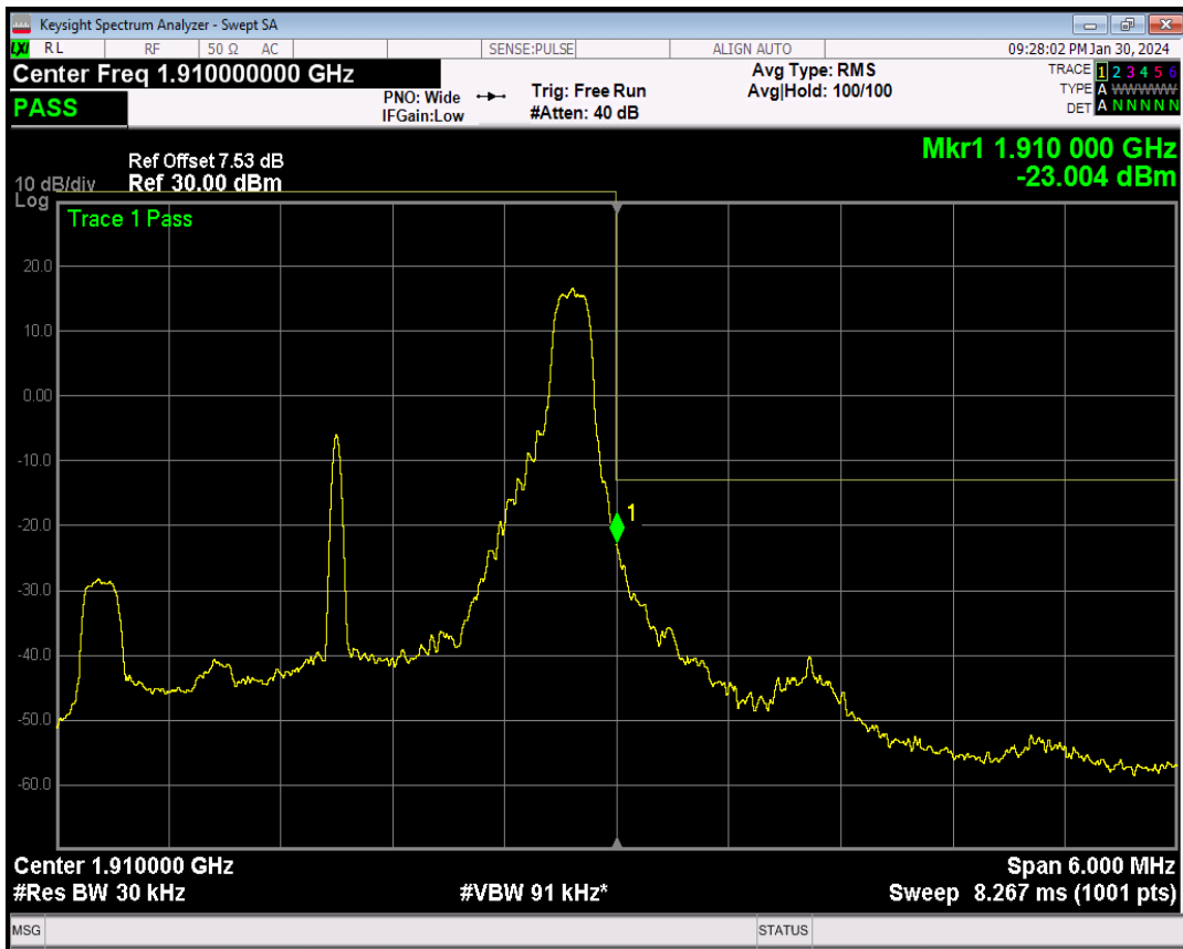
Band2 QPSK BW=3MHz Channel=19185 RB Size=15 Position=#0
