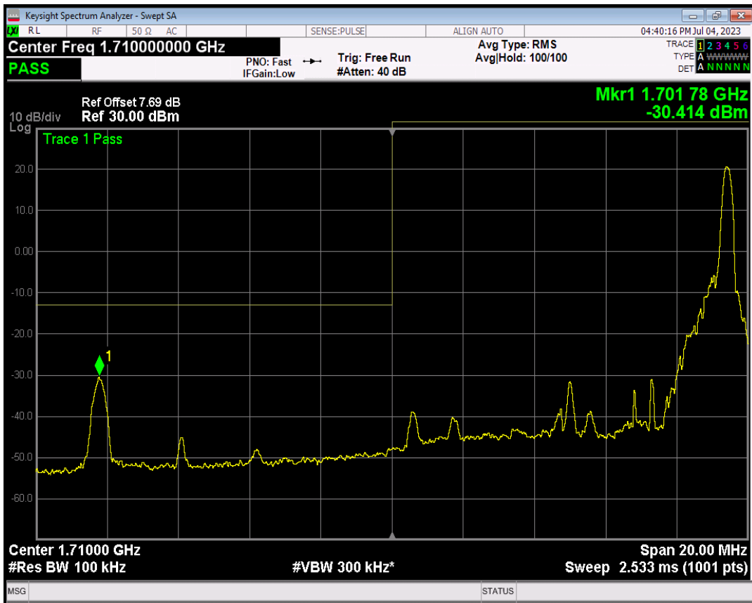
Band4 16QAM BW=10MHz Channel=20000 RB Size=50 Position=#0
