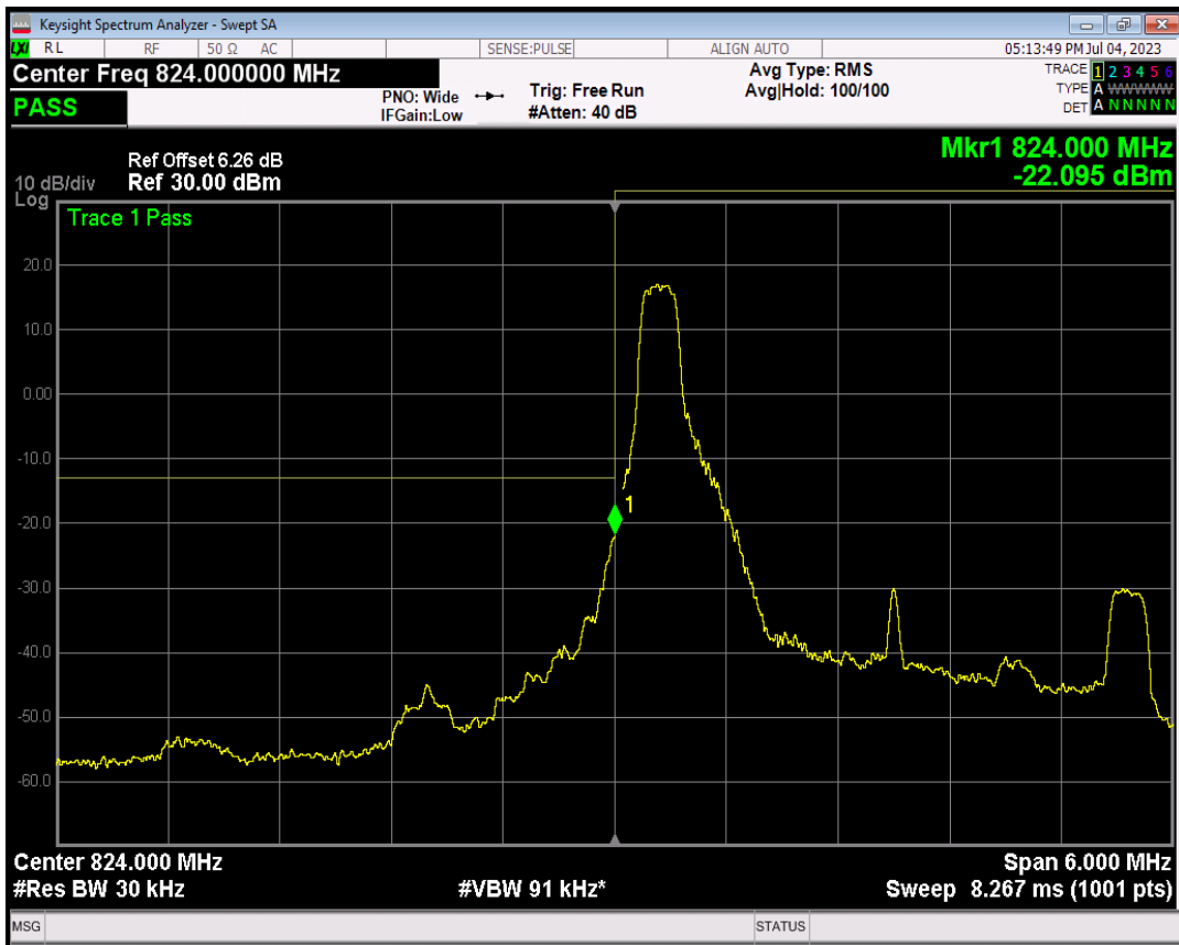
Band5 QPSK BW=3MHz Channel=20415 RB Size=1 Position=#Max
