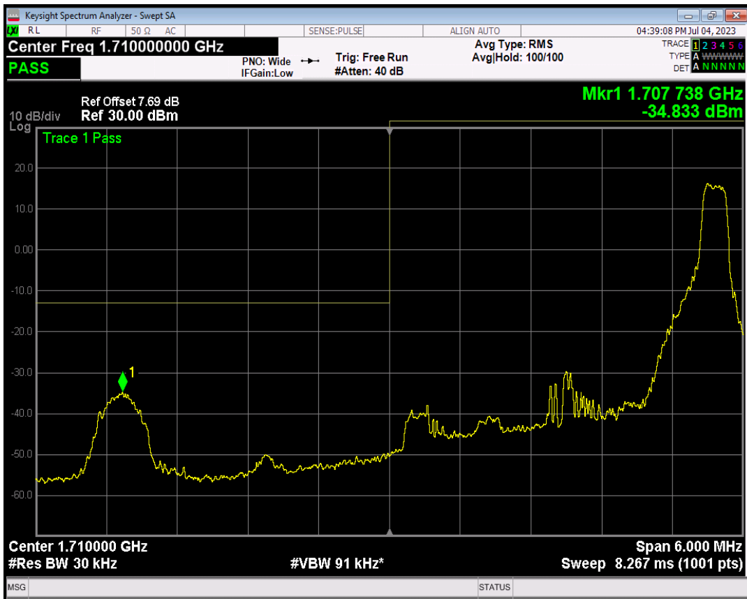
Band4 16QAM BW=3MHz Channel=19965 RB Size=15 Position=#0
