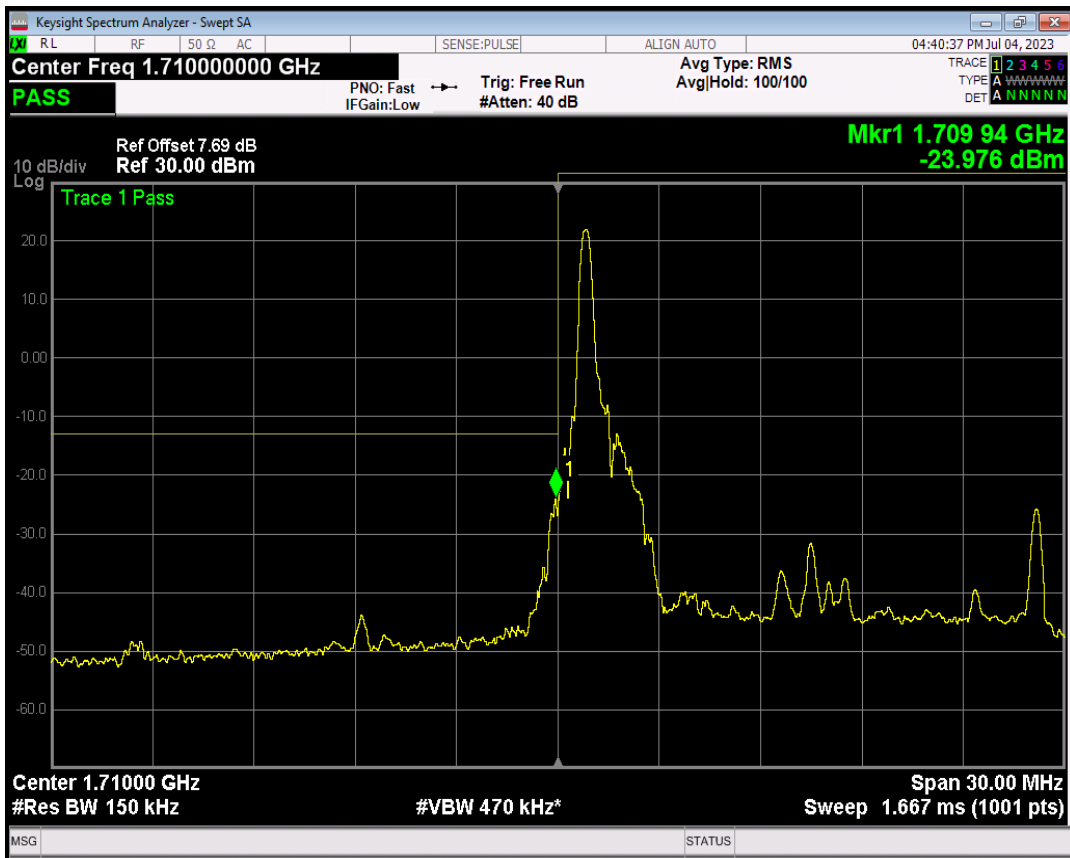
Band4 QPSK BW=15MHz Channel=20025 RB Size=1 Position=#Max
