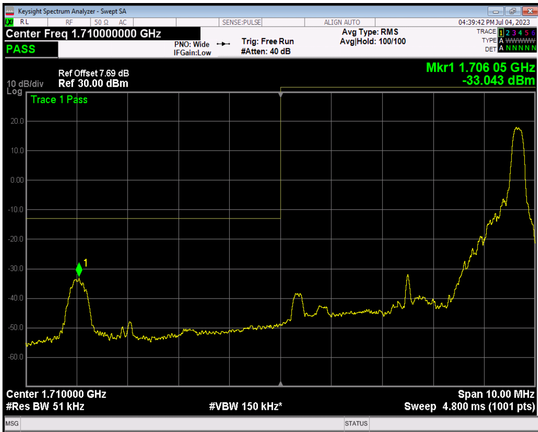
Band4 16QAM BW=5MHz Channel=19975 RB Size=25 Position=#0
