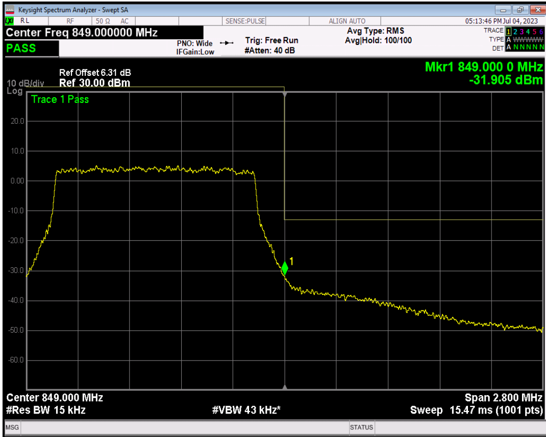
Band5 QPSK BW=3MHz Channel=20415 RB Size=1 Position=#0
