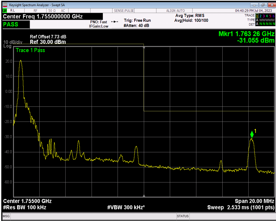
Band4 16QAM BW=10MHz Channel=20350 RB Size=1 Position=#Max
