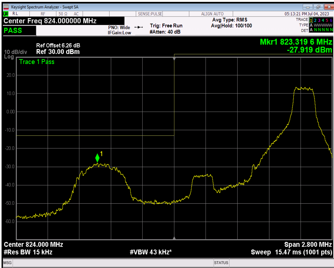
Band5 16QAM BW=1.4MHz Channel=20407 RB Size=6 Position=#0
