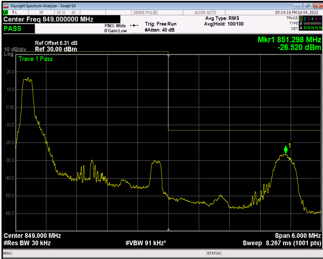
Band5 16QAM BW=3MHz Channel=20635 RB Size=1 Position=#Max
