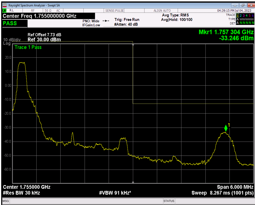
Band4 QPSK BW=3MHz Channel=20385 RB Size=1 Position=#Max
