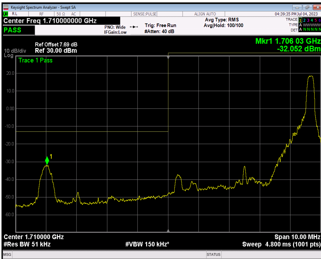
Band4 QPSK BW=5MHz Channel=19975 RB Size=25 Position=#0
