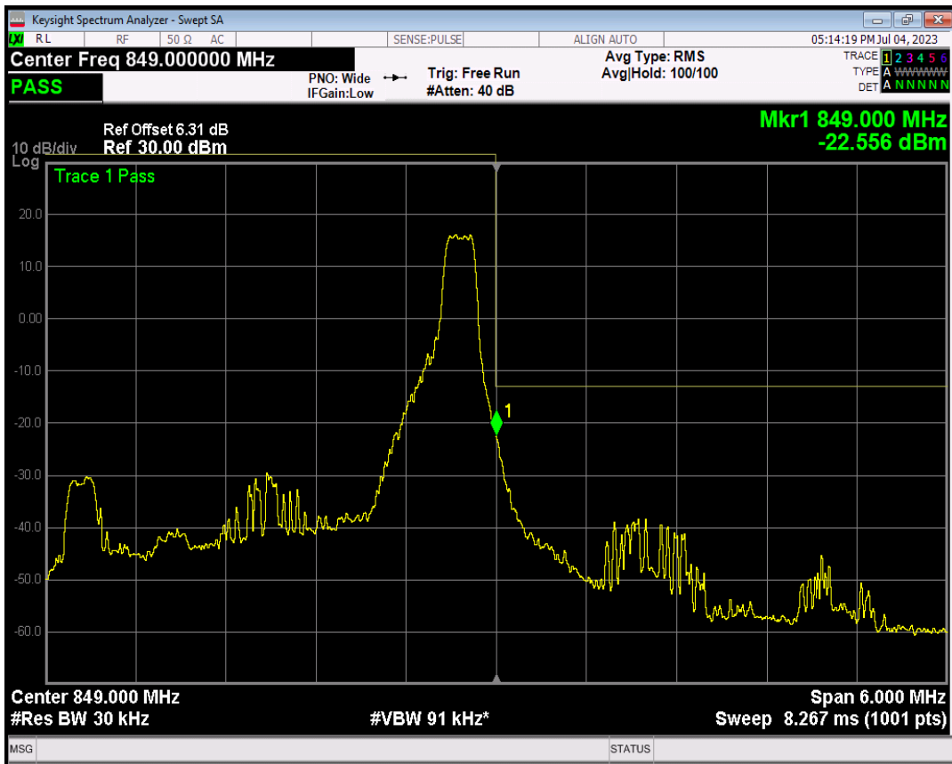
Band5 16QAM BW=3MHz Channel=20635 RB Size=15 Position=#0
