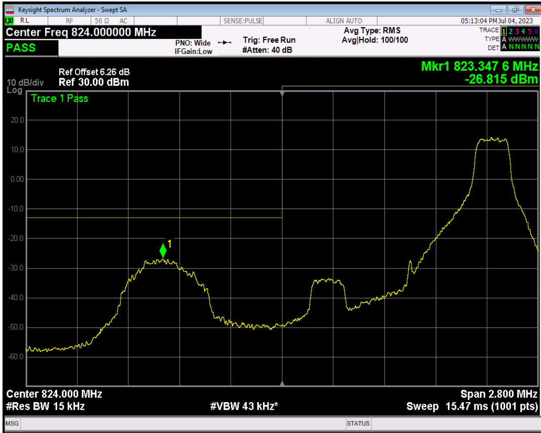
Band5 QPSK BW=1.4MHz Channel=20407 RB Size=6 Position=#0
