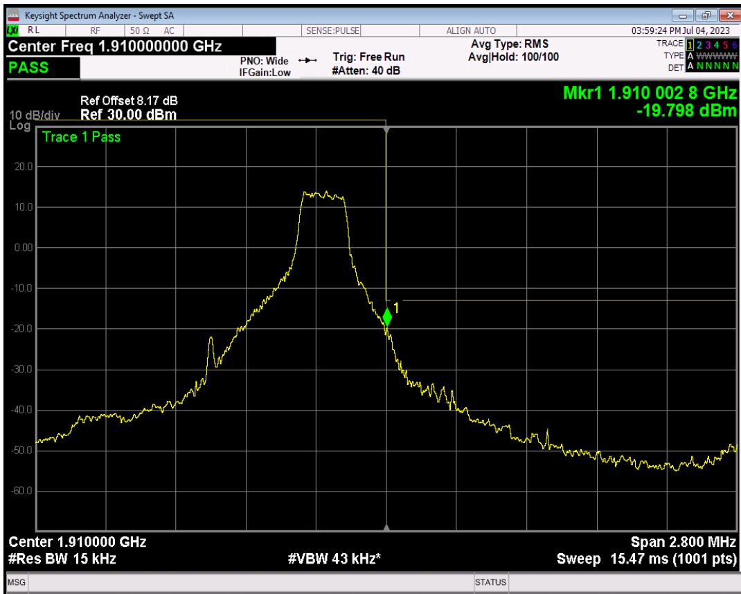
Band2 16QAM BW=1.4MHz Channel=19193 RB Size=6 Position=#0
