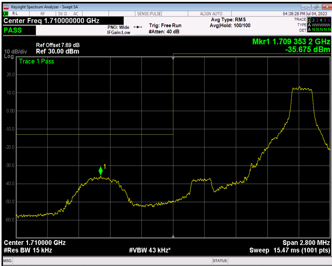
Band4 16QAM BW=1.4MHz Channel=19957 RB Size=6 Position=#0
