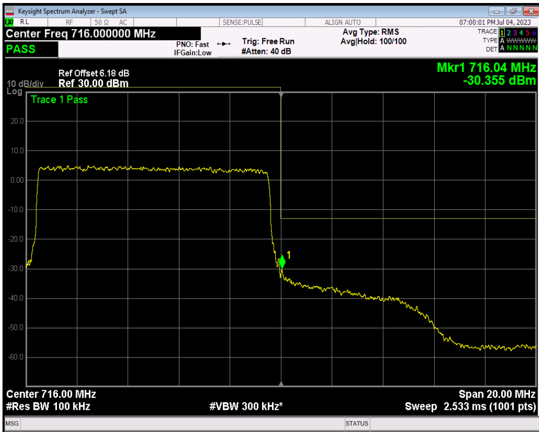
Band17 16QAM BW=10MHz Channel=23800 RB Size=1 Position=#0
