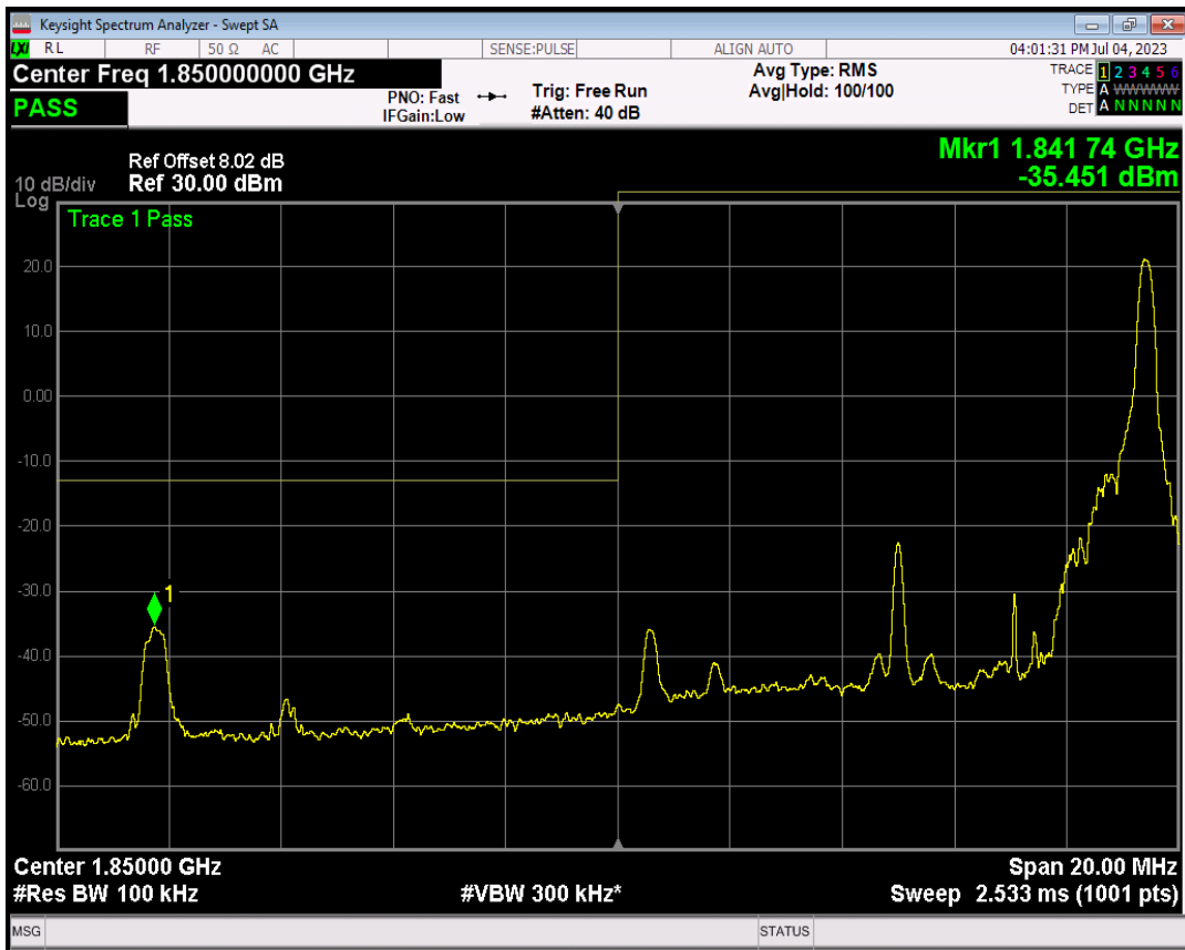
Band2 16QAM BW=10MHz Channel=18650 RB Size=50 Position=#0
