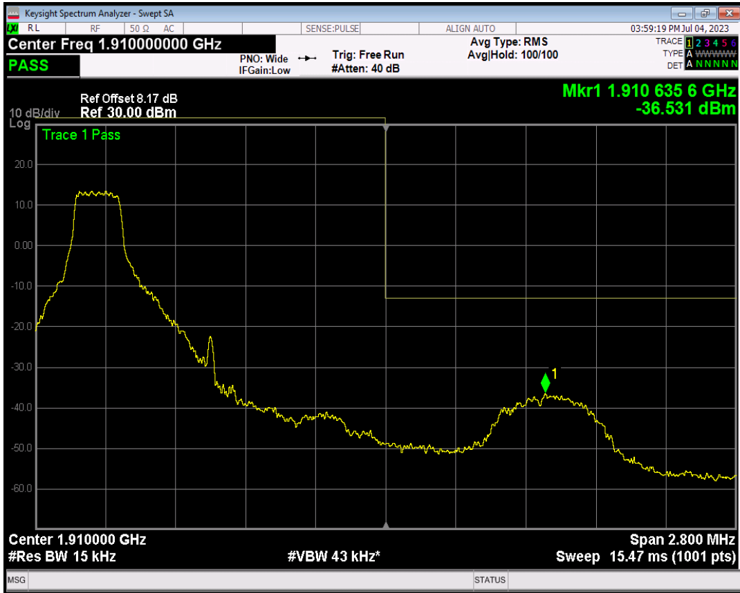
Band2 16QAM BW=1.4MHz Channel=19193 RB Size=1 Position=#Max
