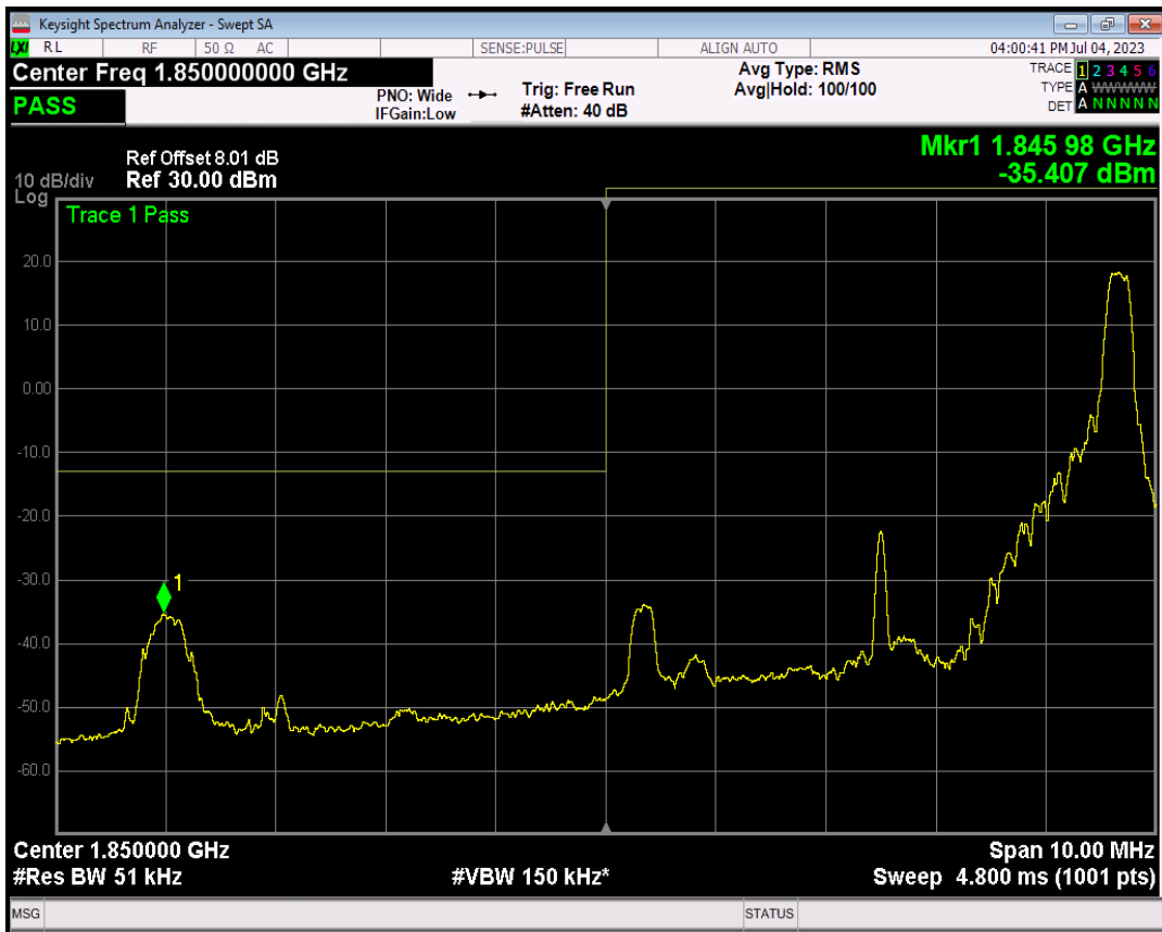
Band2 16QAM BW=5MHz Channel=18625 RB Size=25 Position=#0
