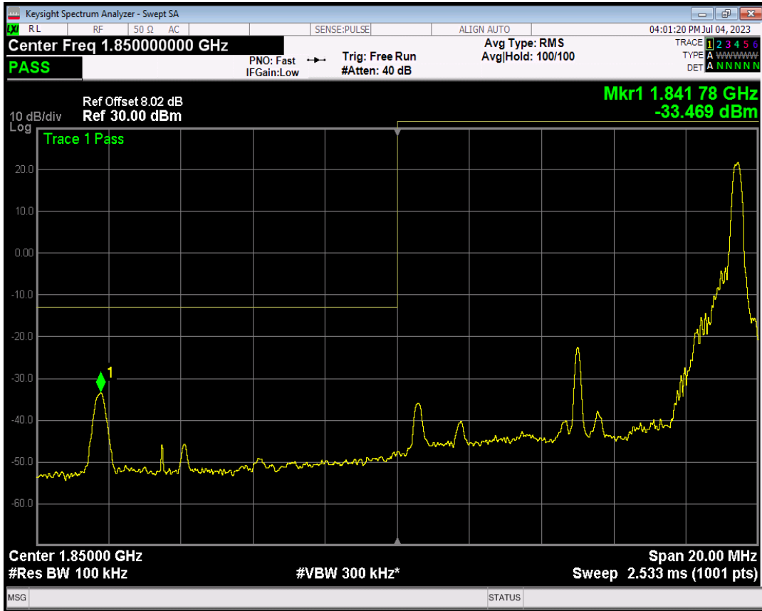
Band2 QPSK BW=10MHz Channel=18650 RB Size=50 Position=#0
