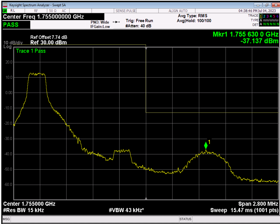
Band4 16QAM BW=1.4MHz Channel=20393 RB Size=1 Position=#Max
