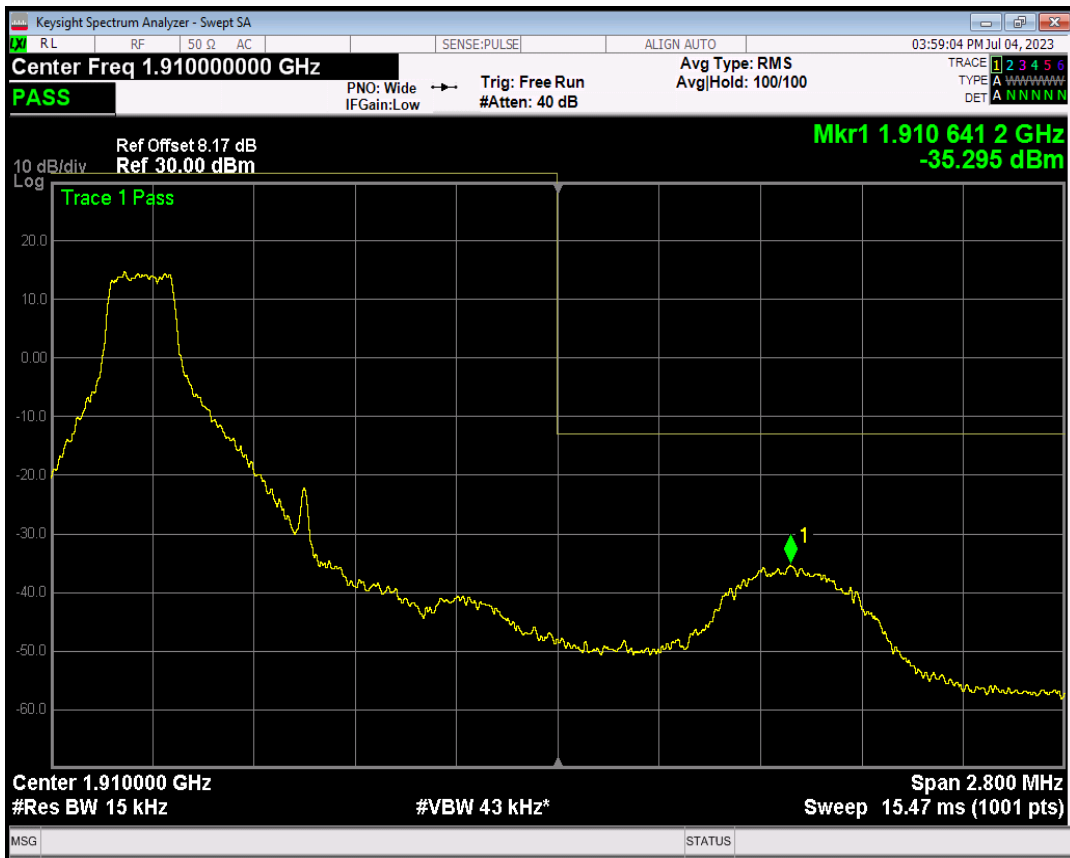
Band2 QPSK BW=1.4MHz Channel=19193 RB Size=1 Position=#Max
