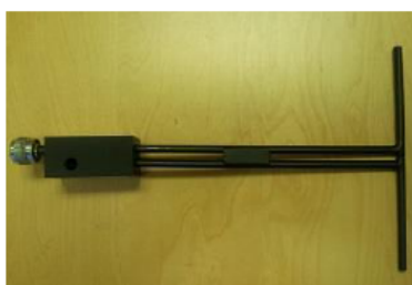
Figure 1 – MVG COMOSAR Validation Dipole
