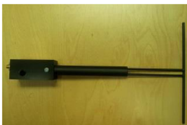
Figure 1 – MVG COMOSAR Validation Dipole
