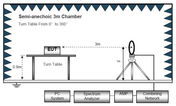
(B) Radiated Emission Test-Up Frequency 30MHz~1GHz
