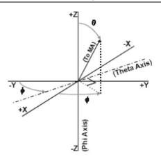
Figure 1 Test coordinate system
