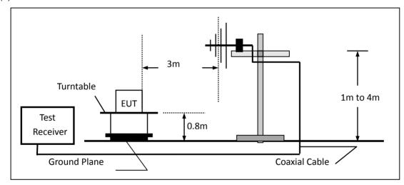
(c) For radiated emissions above 1000MHz
