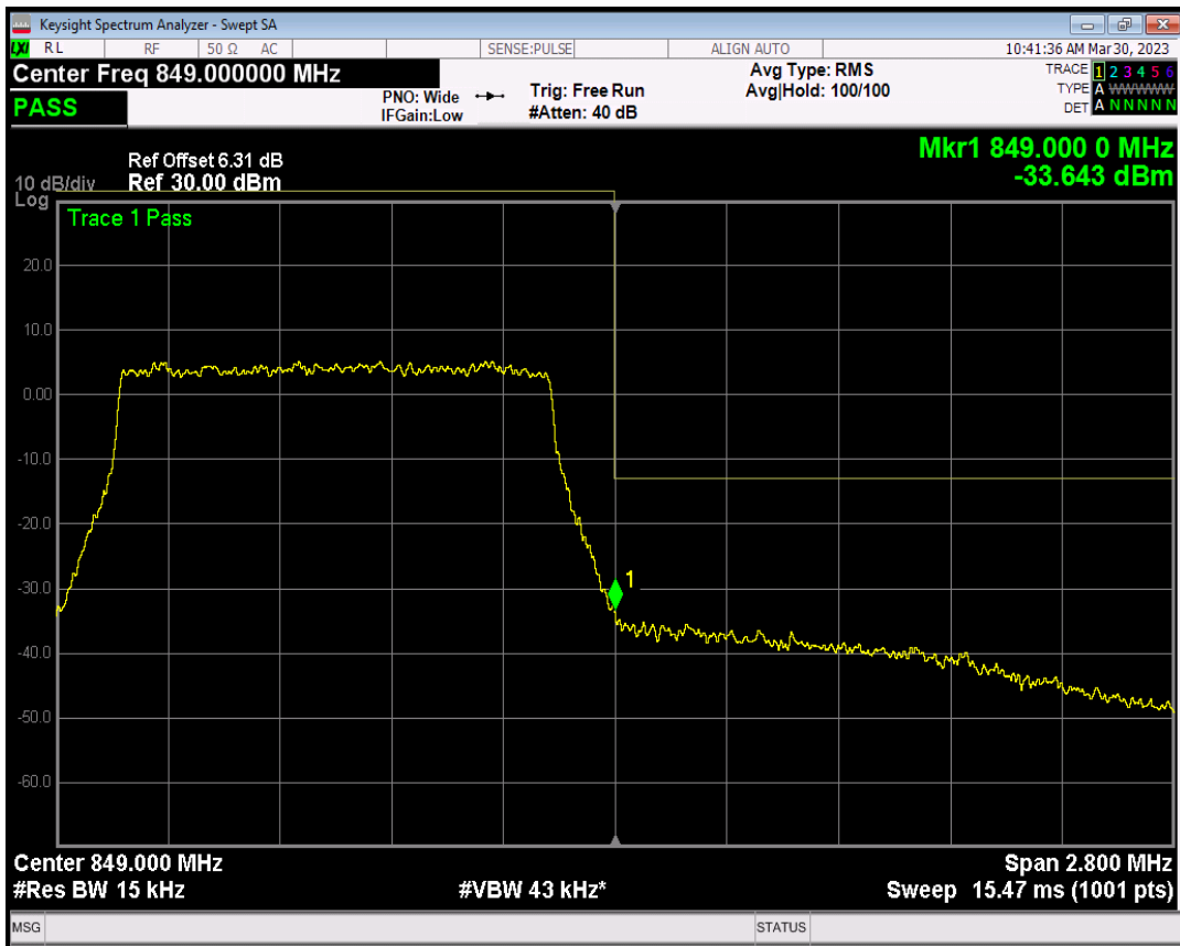
Band5 QPSK BW=3MHz Channel=20415 RB Size=1 Position=#0
