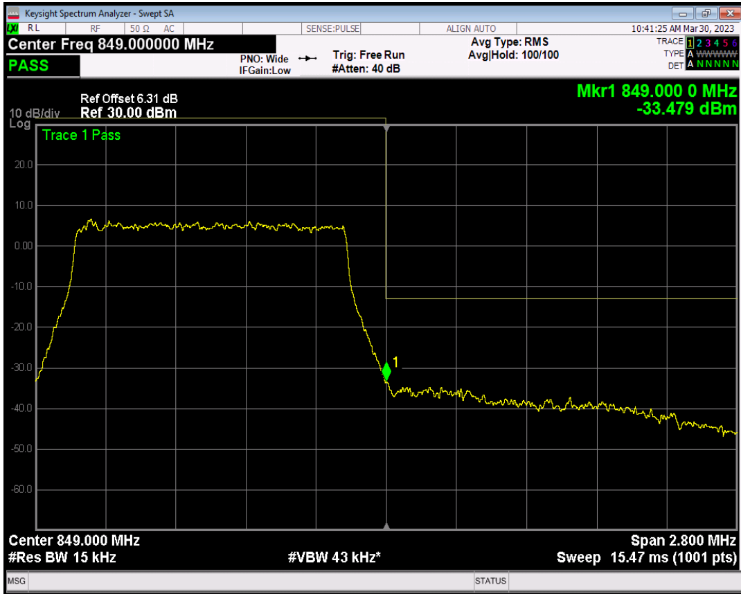
Band5 QAM16 BW=1.4MHz Channel=20643 RB Size=1 Position=#0
