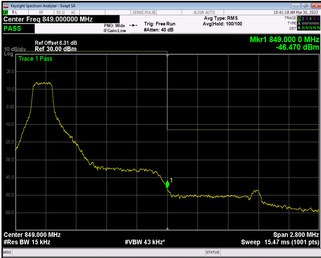
Band5 QPSK BW=1.4MHz Channel=20643 RB Size=1 Position=#Max
