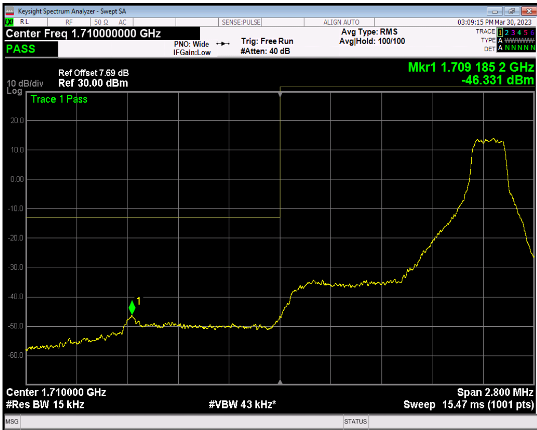
Band66 QPSK BW=1.4MHz Channel=131979 RB Size=6 Position=#0
