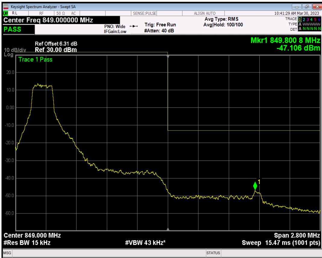
Band5 QAM16 BW=1.4MHz Channel=20643 RB Size=1 Position=#Max
