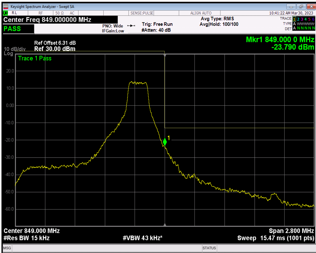
Band5 QPSK BW=1.4MHz Channel=20643 RB Size=6 Position=#0
