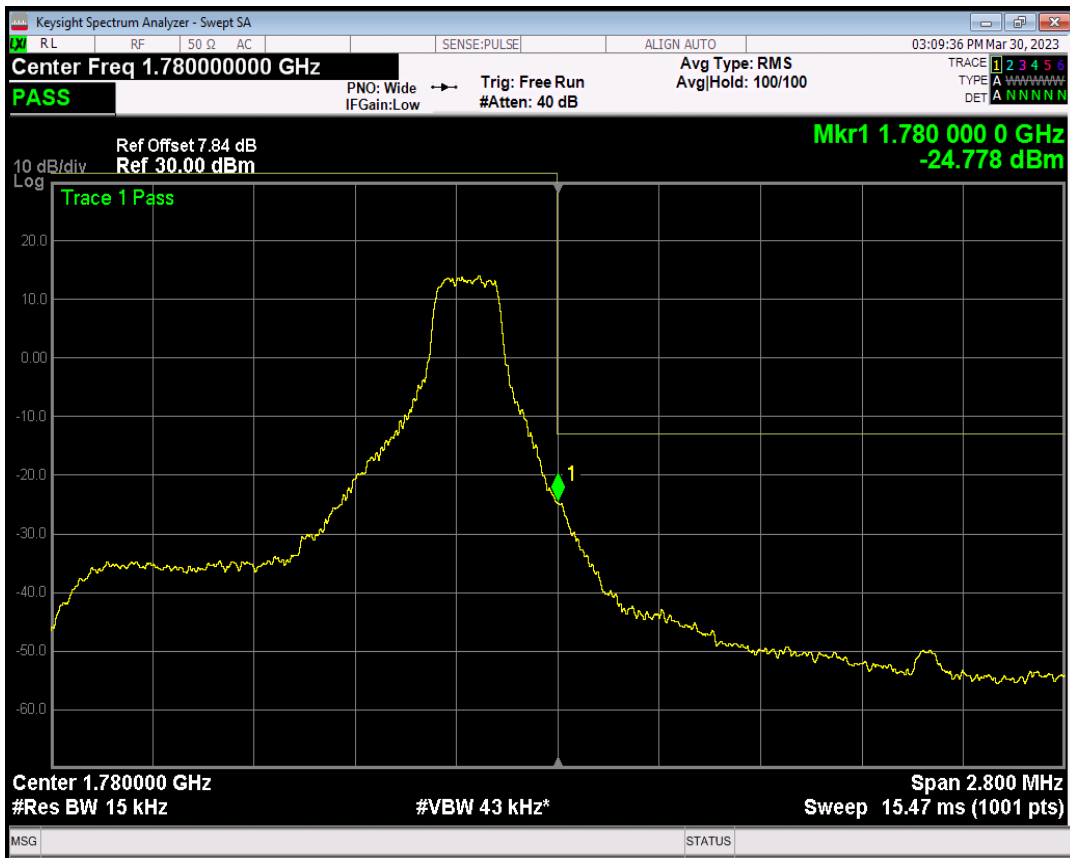
Band66 QPSK BW=1.4MHz Channel=132665 RB Size=6 Position=#0
