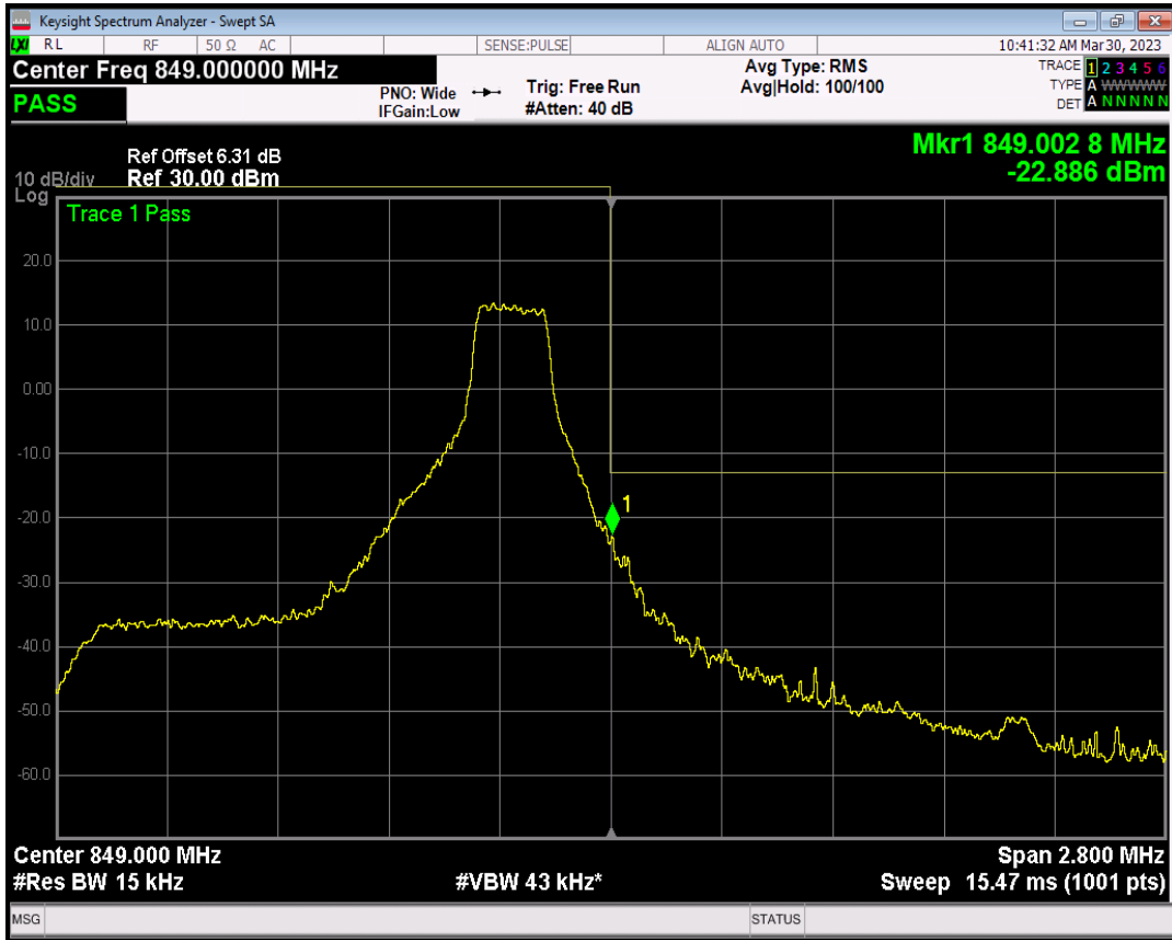
Band5 QAM16 BW=1.4MHz Channel=20643 RB Size=6 Position=#0
