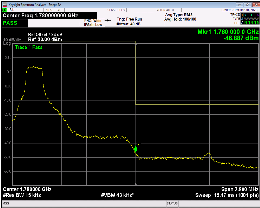
Band66 QPSK BW=1.4MHz Channel=132665 RB Size=1 Position=#Max
