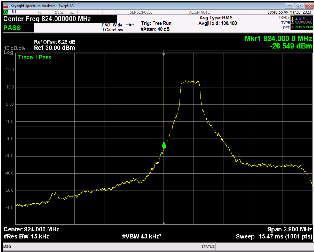
Band5 QPSK BW=1.4MHz Channel=20407 RB Size=1 Position=#Max
