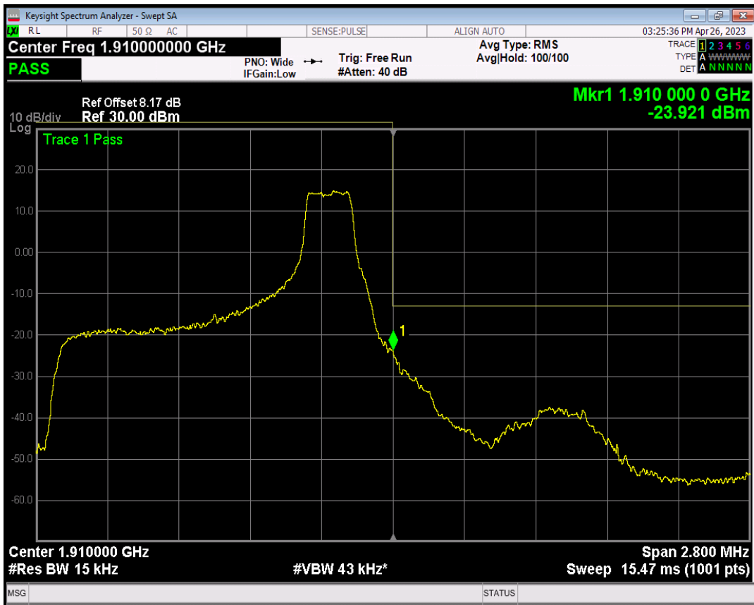
Band2 QPSK BW=1.4MHz Channel=19193 RB Size=6 Position=#0
