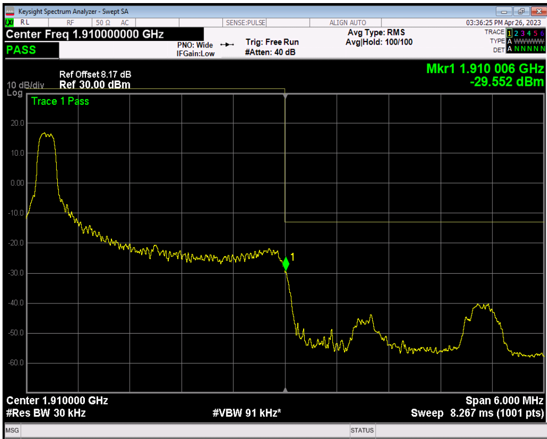
Band2 16QAM BW=3MHz Channel=19185 RB Size=1 Position=#Max
