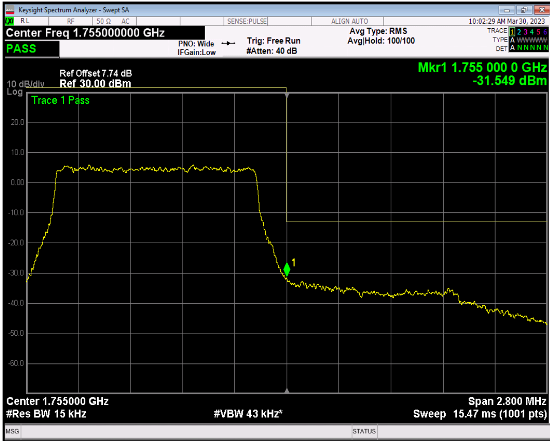
Band4 QAM16 BW=1.4MHz Channel=20393 RB Size=1 Position=#0
