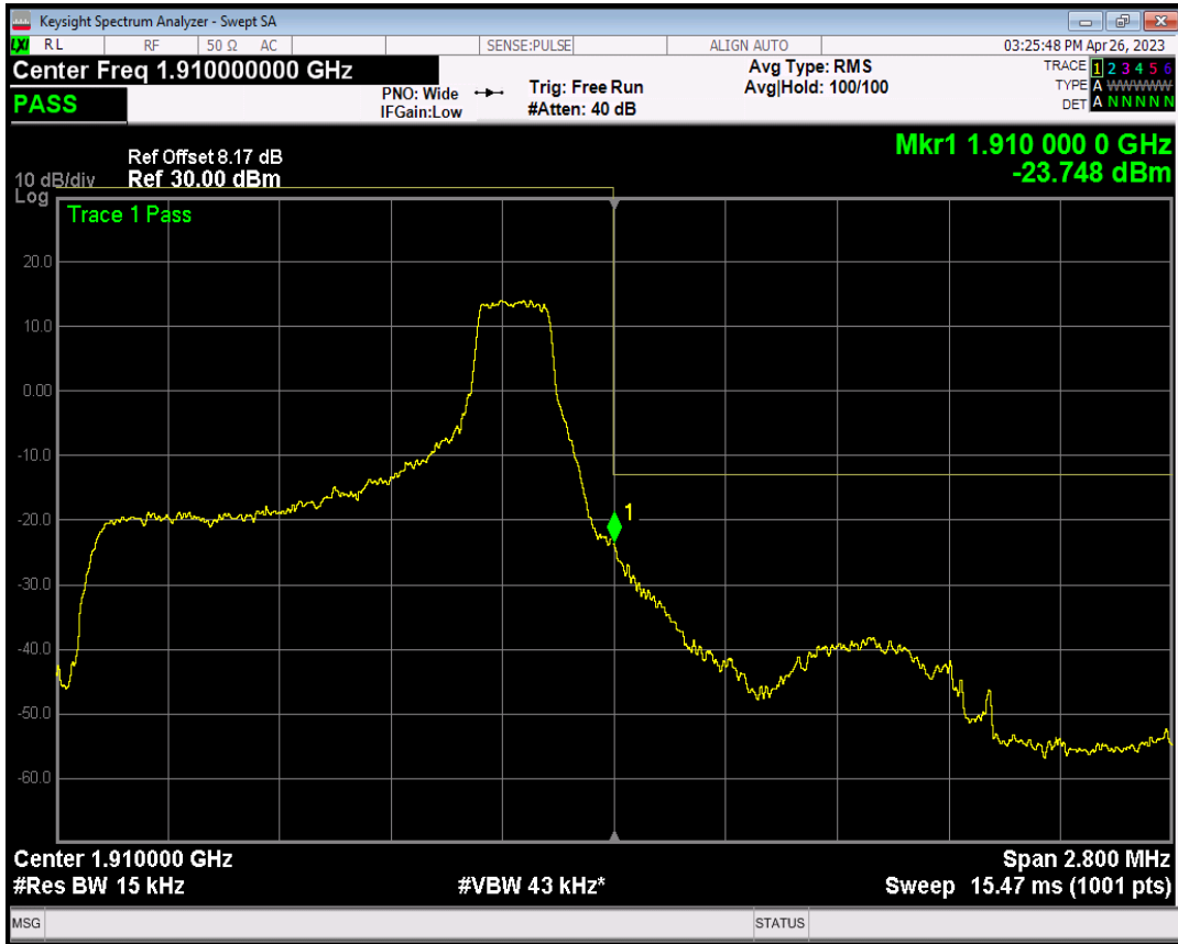
Band2 16QAM BW=1.4MHz Channel=19193 RB Size=6 Position=#0
