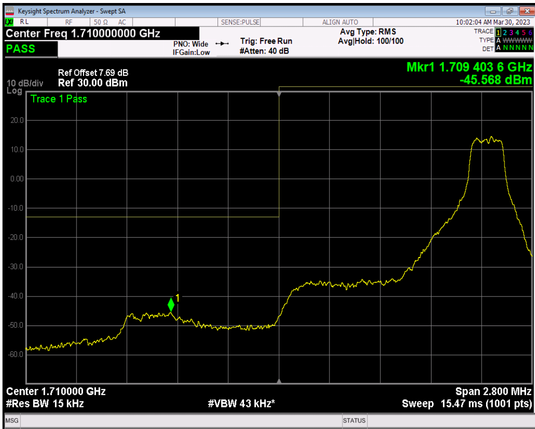
Band4 QPSK BW=1.4MHz Channel=19957 RB Size=6 Position=#0
