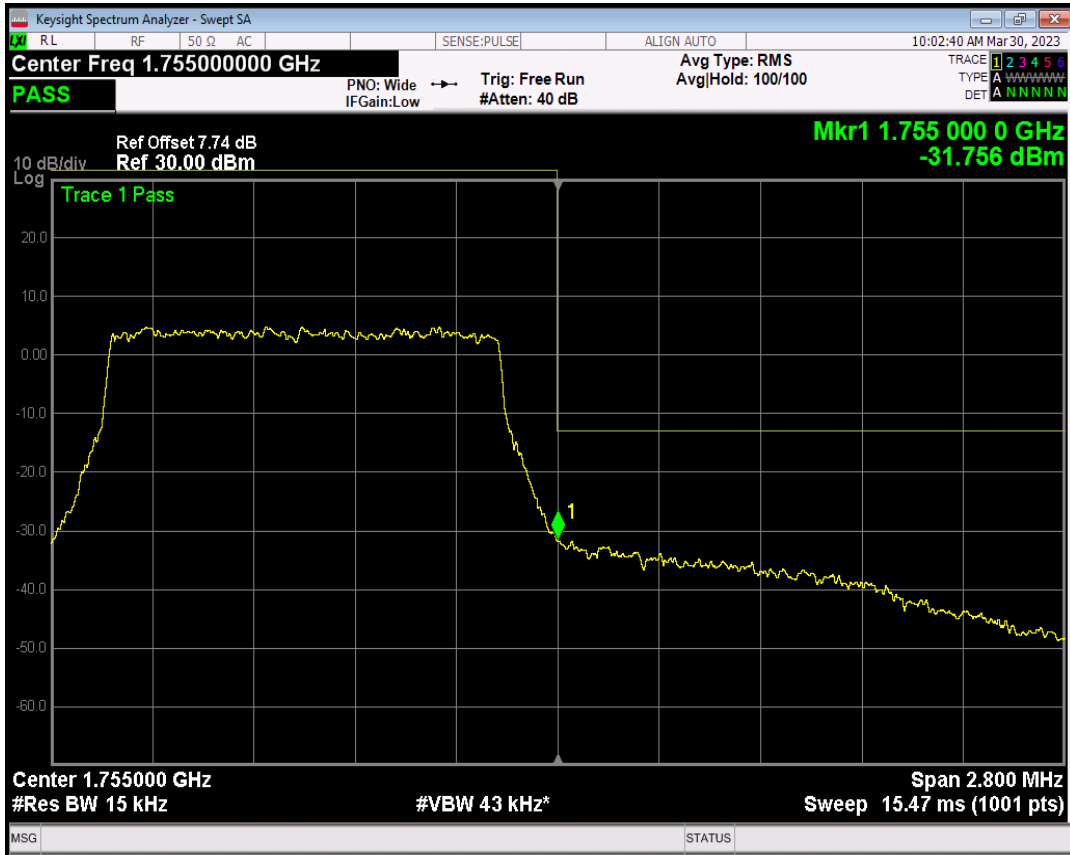
Band4 QPSK BW=3MHz Channel=19965 RB Size=1 Position=#0
