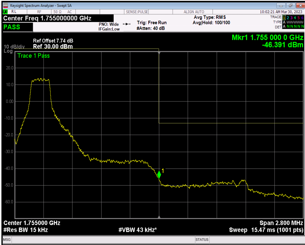
Band4 QPSK BW=1.4MHz Channel=20393 RB Size=1 Position=#Max
