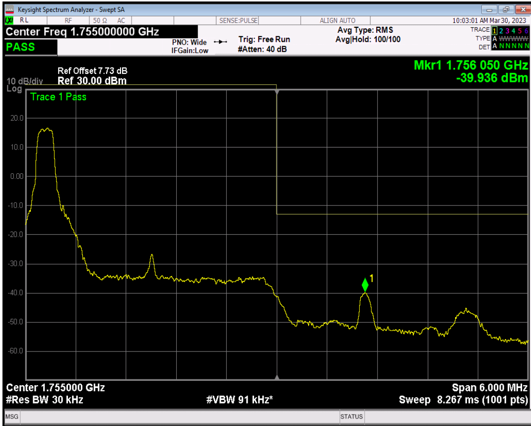
Band4 QPSK BW=3MHz Channel=20385 RB Size=1 Position=#Max
