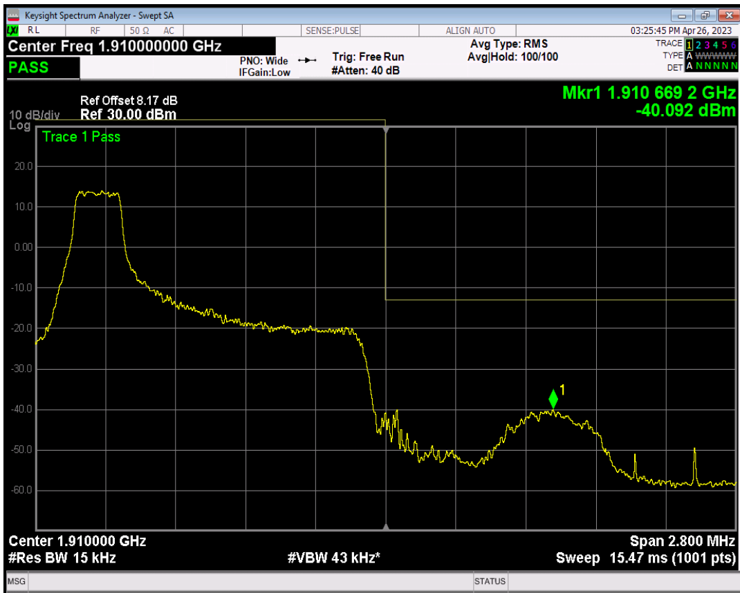
Band2 16QAM BW=1.4MHz Channel=19193 RB Size=1 Position=#Max
