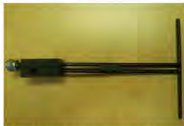
Figure 1 – MVG COMOSAR Validation Dipole
