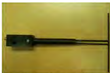
Figure 1 – MVG COMOSAR Validation Dipole
