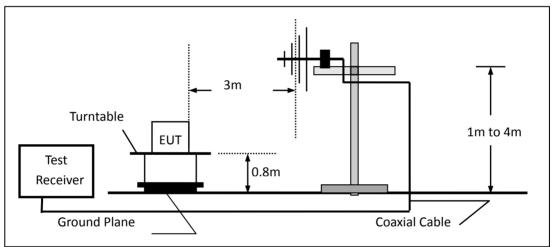
(c) For radiated emissions above 1000MHz
