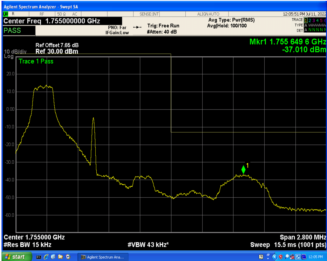
Band4 QAM16 BW=1.4MHz Channel=19957 RB Size=6 Position=#0
