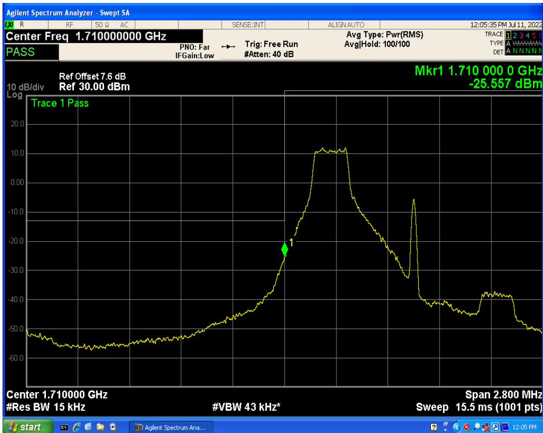
Band4 QPSK BW=1.4MHz Channel=19957 RB Size=6 Position=#0
