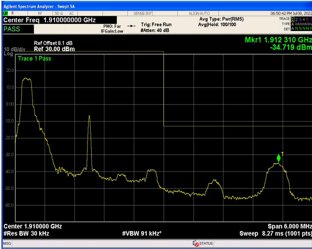
Band2 QPSK BW=3MHz Channel=19185 RB Size=15 Position=#0
