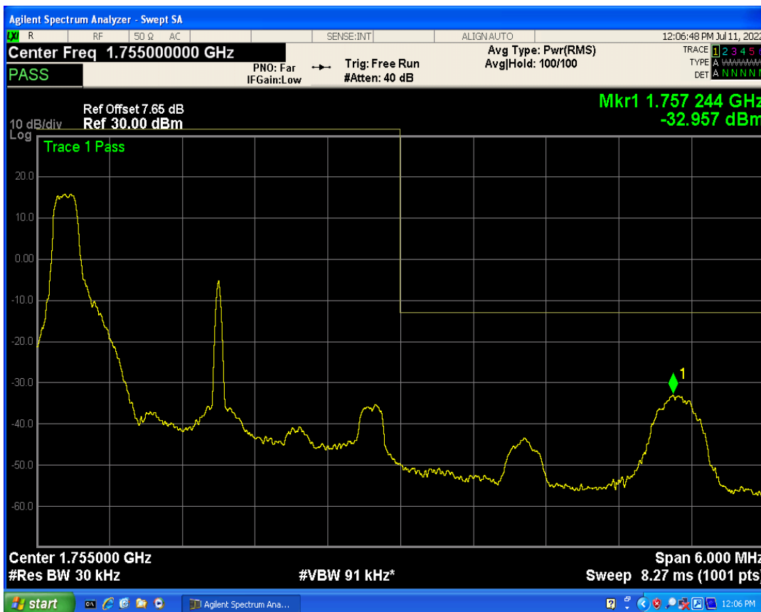
Band4 QAM16 BW=3MHz Channel=19965 RB Size=15 Position=#0
