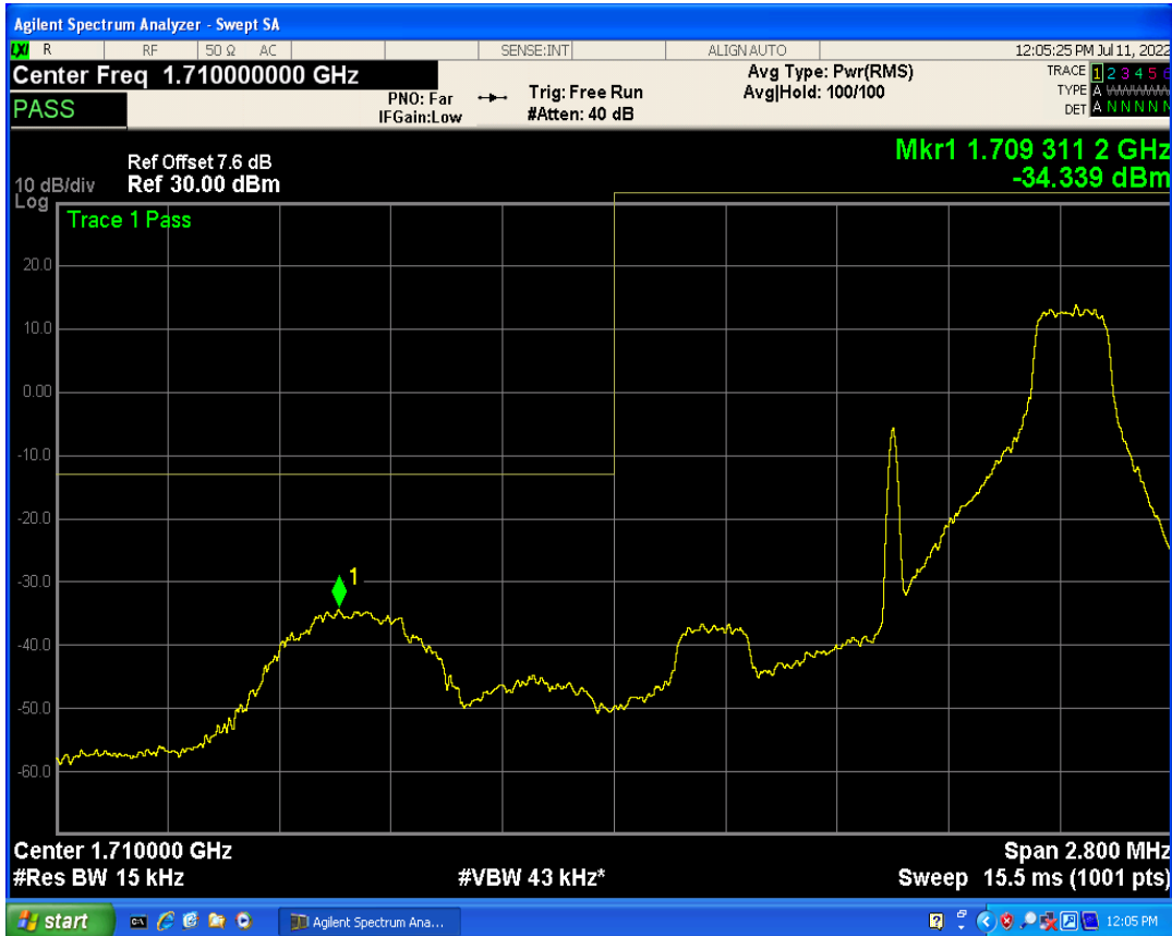
Band4 QAM16 BW=1.4MHz Channel=19957 RB Size=1 Position=#0
