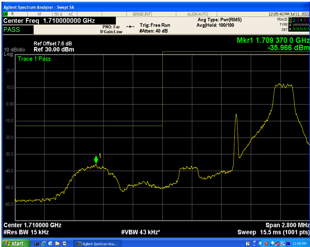
Band4 QPSK BW=1.4MHz Channel=20393 RB Size=1 Position=#0
