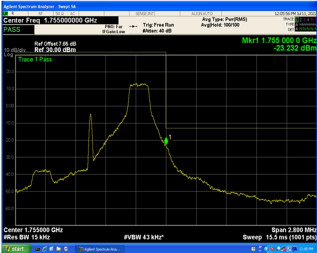
Band4 QPSK BW=1.4MHz Channel=20393 RB Size=6 Position=#0
