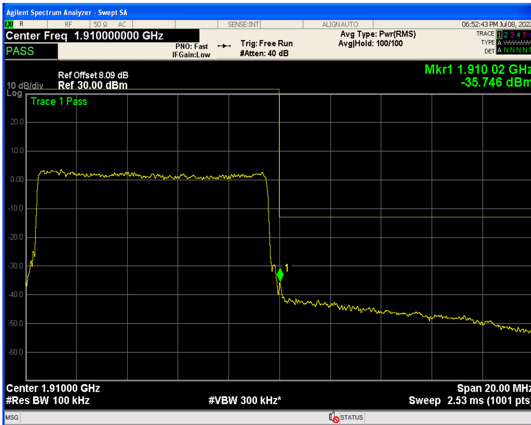
Band2 QPSK BW=15MHz Channel=18675 RB Size=1 Position=#Max
