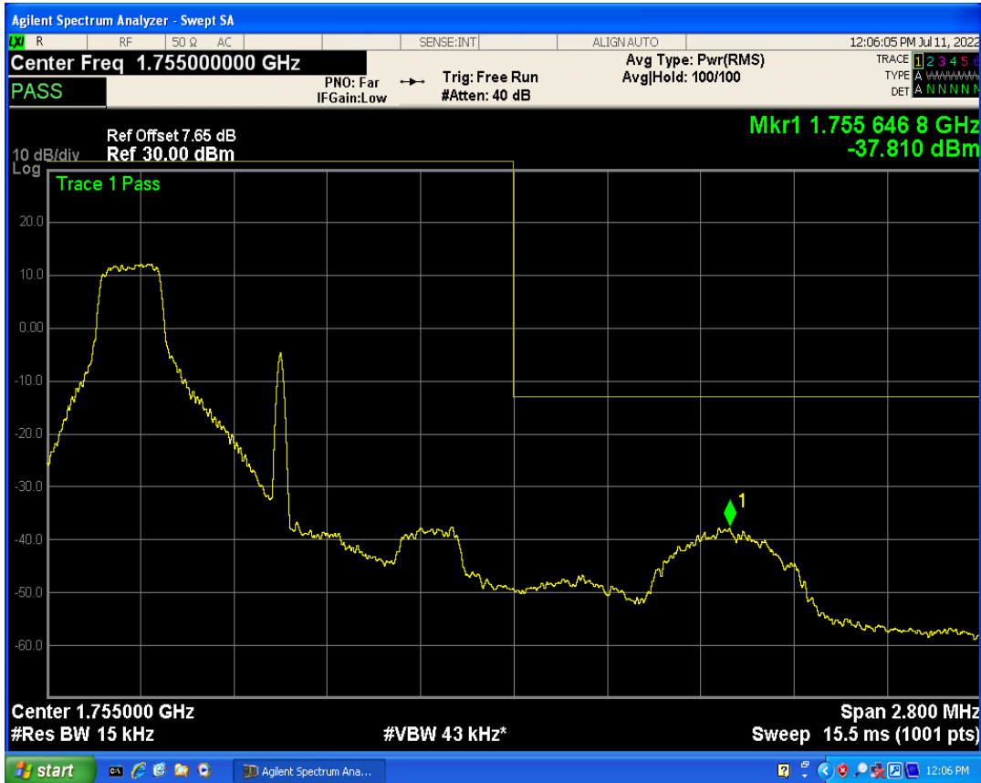
Band4 QAM16 BW=1.4MHz Channel=20393 RB Size=1 Position=#Max
