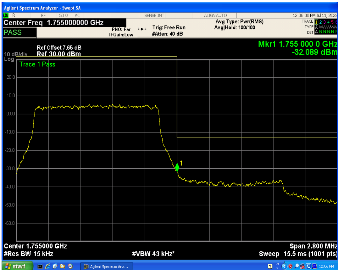
Band4 QAM16 BW=1.4MHz Channel=20393 RB Size=1 Position=#0
