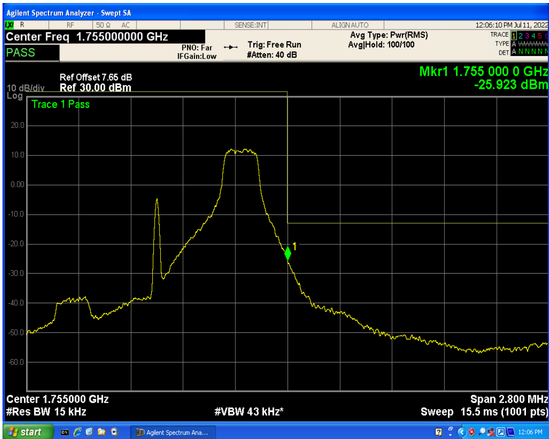
Band4 QPSK BW=3MHz Channel=19965 RB Size=1 Position=#0
